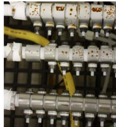
Specimens at 10 g/m 2 (top), 1 g/m 2 (middle), and 0.1 g/m 2 (bottom)
