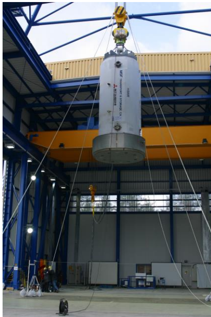
9 m vertical drop test
