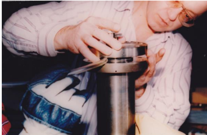
Cs corrosion tests of the lid closures of 9 small heated containers (BAM, 1992)
