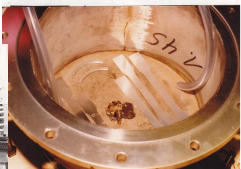
Cs corrosion test of Aluminum and Silicon specimen
