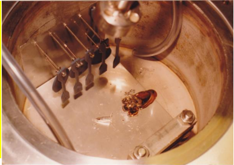
Cs corrosion test of Aluminum and Silicon specimen
