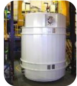
Example of spent fuel transport and storage cask for which license will cover DFR* loaded in capsules: TN ® 24 SH cask
