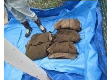
Put residue in burlap sacks. The sacks are folded and stacked on a water sealing sheet
