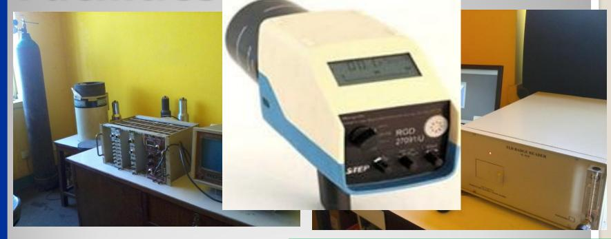
MCA- NaI Detector | TLD | for Environment & Few Survey Meters | Personnel Radiation Calibrating Sources monitoring system
