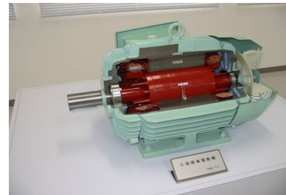
Three-phase Induction Motor
