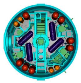
SS rooms are placed from each side of Containment. Middle pressure HAs for VVER-TOI are placed under maintenance floor
