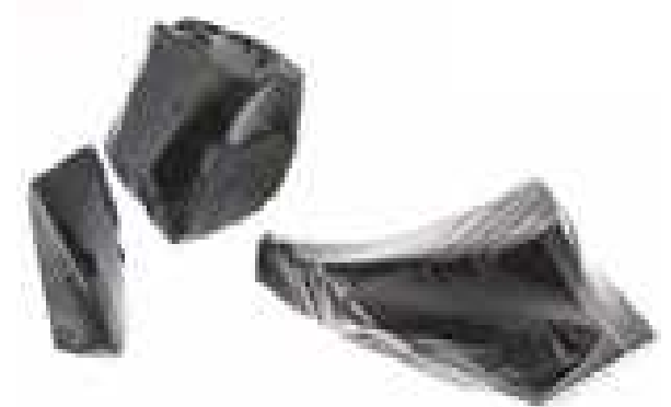
Developing technologies – vitrified waste from Savannah River, South Carolina
