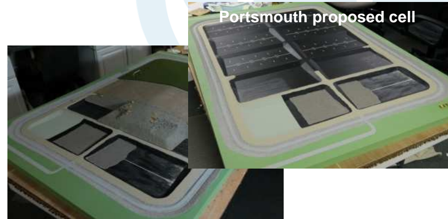
Physical model of proposed disposal facility with removable layers (liner, waste, cover)
