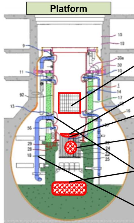
Estimation of damaged core of Unit-1
