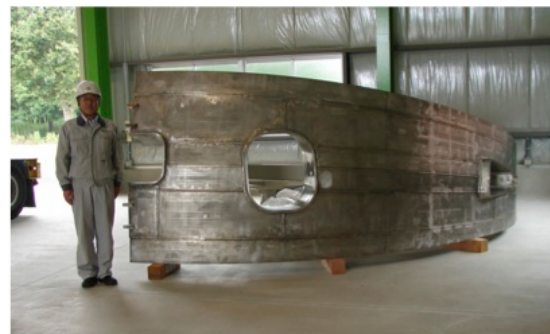
Fig.12 Trial upper half of the 20 degree sector of the vacuum vessel was delivered to the Naka site
