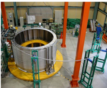
Fig.9 Manufacturing of EF conductors with a 630 m jacketing line at the JAEA Naka Site in May 2010
