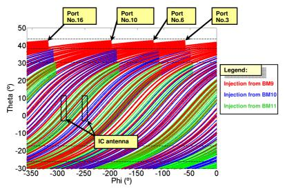
Figure 4 Field line mapping in the poloidal-toroidal plane for varying poloidal injection location at the proposed toroidal injection points. The map has been produced using the most up to date baseline  $Q_{DT} = 10$  magnetic equilibrium.
