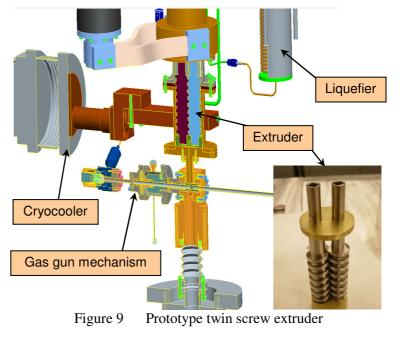
circuit to form the fully integrated prototype pellet injector for ITER [4].
