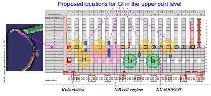
Red boxes are the bolometers, orange the VIS/IR, green the Neutral Particle Analyzer: Interferences are expected in the shaded ellipses. Figure 5 Currently envisaged distribution of physical gas injection points
