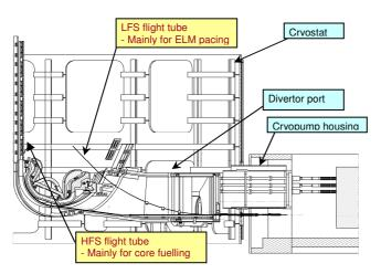
Figure 7 Pellet Flight Tube Layout
