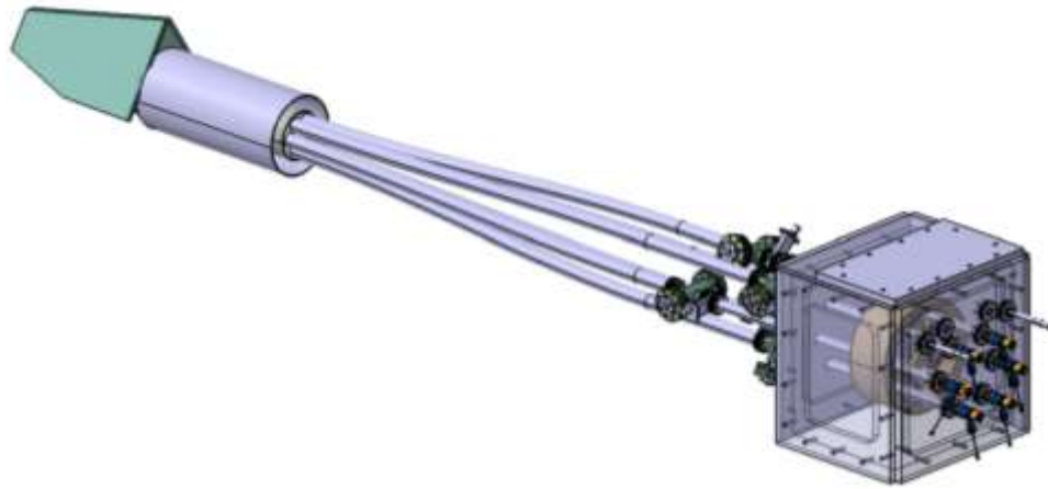
Fig. 4. CAD model of the large diameter 6 barrel pipe-gun device for mitigating disruptions in ITER with large cryogenic pellets that are shattered before entering the plasma. Propellant valves are mounted on the back surface of the injector guard vacuum box. The 6 barrels are tapered to meet at the shatter plate.
