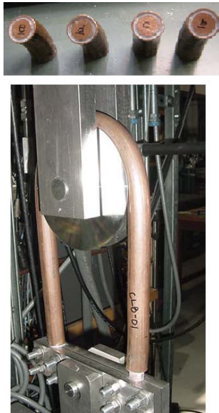
Fig 2 Above: Sections Cut from the U bend test, Below the U-Bend test fixture
