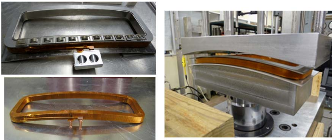
Fig 10 DIII-D CP Coil Components At Left: Coil cover and one of the four strips of Inconel 718 springs, the Bonded Coil At Right, the Preload Assembly Fixture
