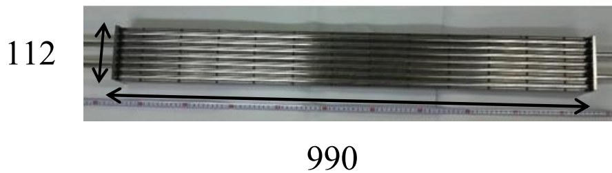
FIG. 8. Appearance of pebble bed container mock-up.
