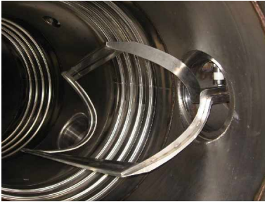
FIG. 9. Frame antenna inside vacuum vessel.
