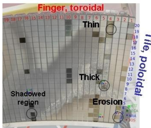
Fig. 1. Part of the toroidal pump limiter of Tore Supra. The numbers denoting the tile position and different deposition regions are marked.
