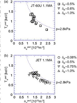
FIG. 5. (a) The pedestal n-T diagram for the cases before and after the installation of FSTs in JT-60U at 1.1MA. (b) The pedestal n-T diagram in JET TF ripple scan experiment at 1.1MA. Broken curves indicate a constant electron pressure of 2.8kPa.
