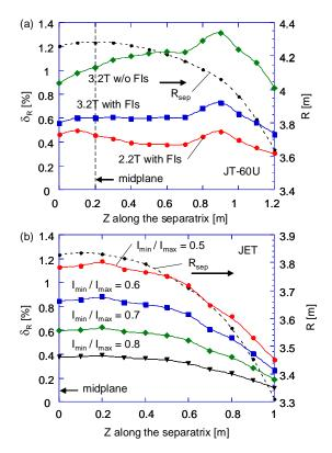
FIG. 3. The local TF ripple value as a function of Z value along the separatrix in the configuration for the similarity experiment using (a) JT-60U and (b) JET TF coil system.  $I_{min}/I_{max}$ denotes the ratio of odd to even number of TF coils in JET. The R value at the separatrix gradually becomes smaller with increasing Z value.
