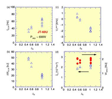
FIG. 8. Dependence of (a)ELM frequency, (b) ELM energy loss, (c) pedestal toroidal rotation frequency, (d) line-averaged electron density, and total stored energy on the TF ripple amplitude in JT-60U.
