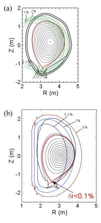
FIG. 1. Plasma cross sections for the similarity experiments together with TF ripple amplitude  $\delta_R$  in (a) JT-60U and (b) JET. Here,  $\delta_R$  is defined as  $(B_{TMax} - B_{TMin})/(B_{TMax} + B_{TMin})$ . The number of TF coils is 18 in JT-60U and 32 in JET.
