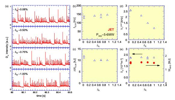
FIG. 9. (a)  $D_{\alpha}$  emission intensity at the outer divertor for the variation of TF ripple in JET. Dependence of TF ripple on (b) ELM frequency, (c) ELM energy loss, (d) edge toroidal rotation frequency, (e) line-averaged electron density, and total stored energy.
