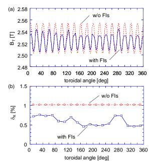
FIG. 2. (a) The  $B_T$  along the toroidal angle at the separatrix on the outer midplane (R=4.28m, Z=0.2m) for the cases before and after the installation of FIs in JT-60U. (b) The TF ripple at each section between 2 TF coils.
