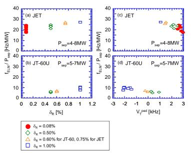
FIG. 10. ELM frequency normalized to the power crossing the separatrix observed in JET and JT-60U as a function of  $\delta_{R}$  and  $V_{T}^{ped}$ .
