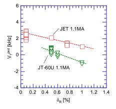
FIG. 4. The toroidal rotation velocity at the H-mode pedestal shoulder  $V_T^{ped}$  as a function of  $\delta_R$ . Squares and inverse triangles indicate the data taken from the similarity experiment at 1.1MA in JET and JT-60U, respectively. The TF ripple scan conducted using the JET standard configuration at 2.6MA is also plotted as triangles for reference.
