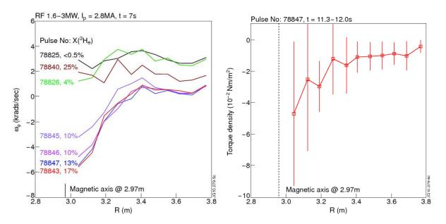
Figure 3. (Left frame) Toroidal rotation profiles from  $I_p=2.8$  MA pulses at different He<sup>3</sup> concentration levels. Negative  $\omega_{\phi}$  is defined as in the counter- $I_p$  direction. (Right frame) Estimated torque density profile from pulse no. 78847 with  $P_{ICRH}=1.8$  MW and He<sup>3</sup> concentration = 13%. The separatrix is at  $R_{sep}\approx3.90$ m and magnetic axis at  $R_0\approx2.97$ m for all shots. Reprinted from [16,17].
