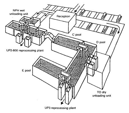
FIG. 15. Spent fuel reception, unloading and storage complex at La Hague, France.
