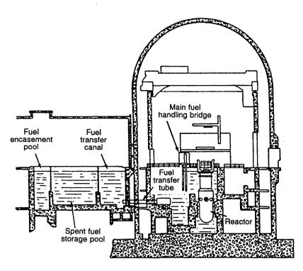
FIG. 5. Cross-section showing the relationship of the PWR core and the spent fuel pool.
