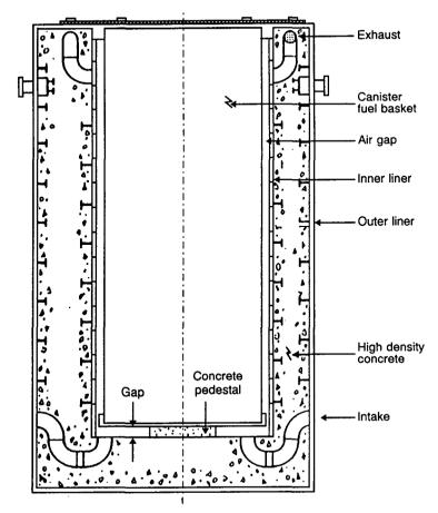
FIG. 8. Conceptual design for a ventilated concrete storage cask.
