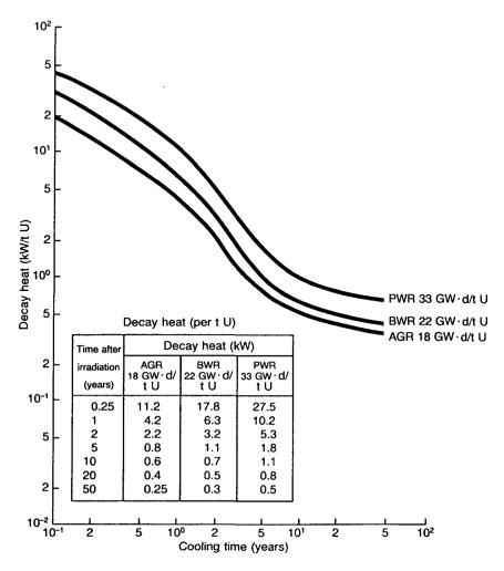
FIG. 2. Thermal (decay heat) output of spent fuel with time.
