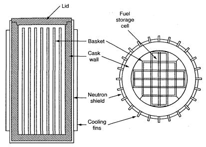
FIG. 6. Conceptual design for a typical metal storage cask.
