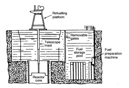
FIG. 4. Cross-section showing the relationship of the BWR core and the spent fuel pool.
