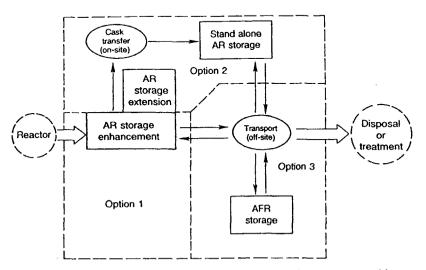
FIG. 3. Three options for the storage of spent fuel (arrowed lines are possible transport operations).
