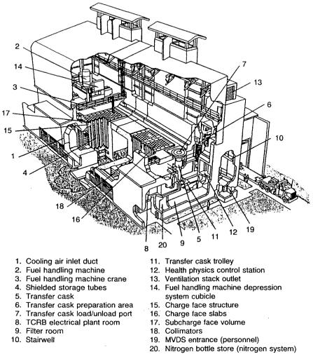
FIG. 9. Cutaway view of the modular vault dry storage (MVDS) system.
