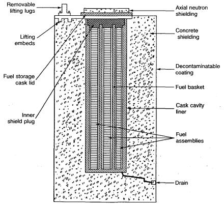
FIG. 7. Conceptual design for an unventilated concrete storage cask.
