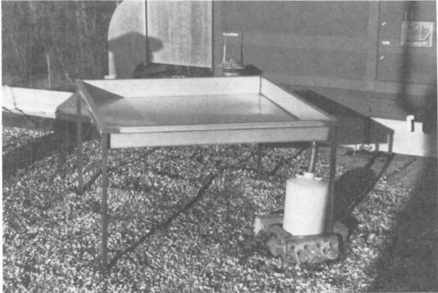
*FIG. 10. Typical rain water collector.*
