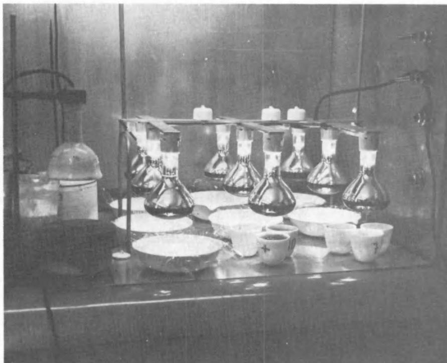
*FIG. 7. Evaporation lamps for drying samples.*
