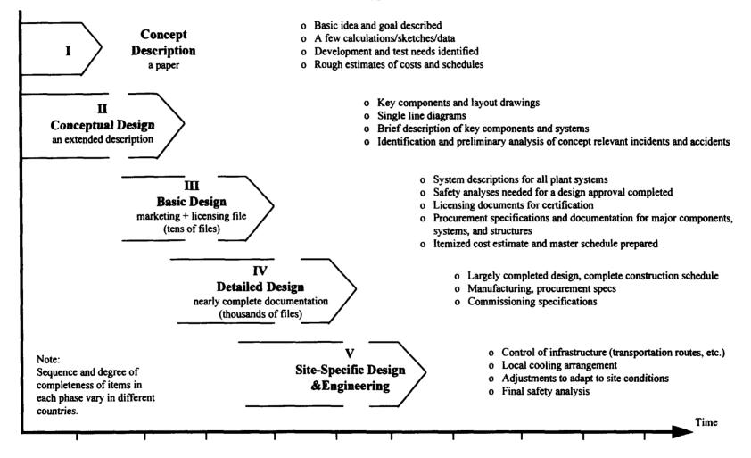
FIG. B1. Phases and corresponding activities during design development (excluding major testing).
