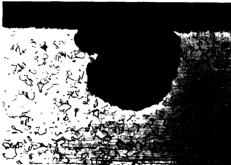
FIG.10 OPTICAL MICROGRAPH OF HASTELLOY C4 AFTER 606 DAYS IMMERSION IN Q-BRINE AT 90° C WITH GAMMA-IRRADIATION ( 10^3 Gy/h)
