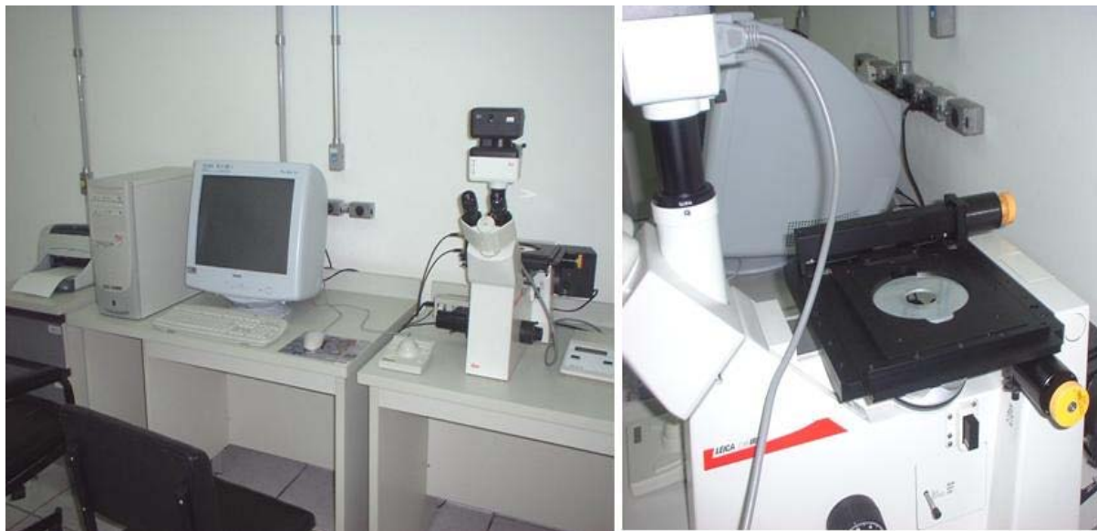
FIG. 8. The Leica Image Analysis Work Station (left) and detail of the motorised stage (right).
