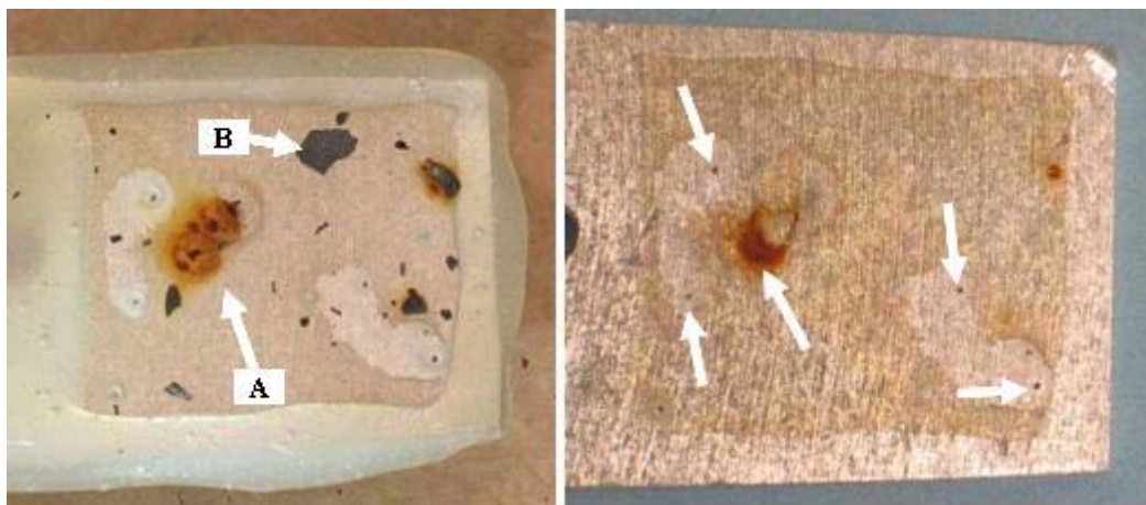
FIG 27. Sample tested with magnetite deposits, before (left) and after (right) cleaning. "A": transformed particle, "B": non-transformed particle. Arrows indicate pitting attack.
