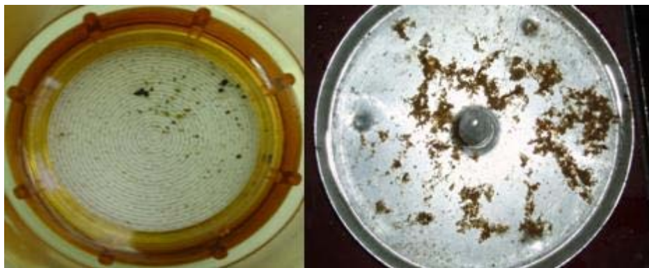
FIG. 16. Settled solids on a millipore filter (left) and the collector (right).
