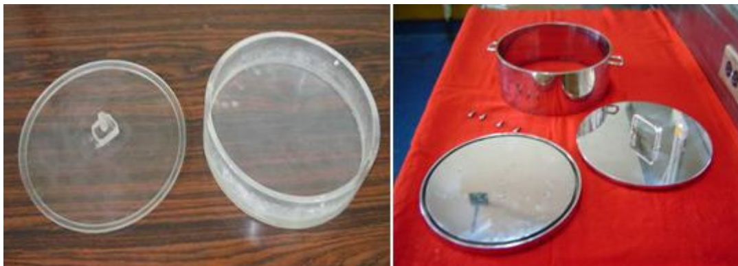
FIG. 13. Collectors used in: (left) CDTN, Brazil. Material: Acrylic, Dimensions: diameter: 18.9 cm, height: 3.8 cm, Area: 280.6 cm 2 . (right) IPEN, Peru. Material: Aluminium, Dimensions: Diameter: 20 cm; Area: 314 cm 2 .
