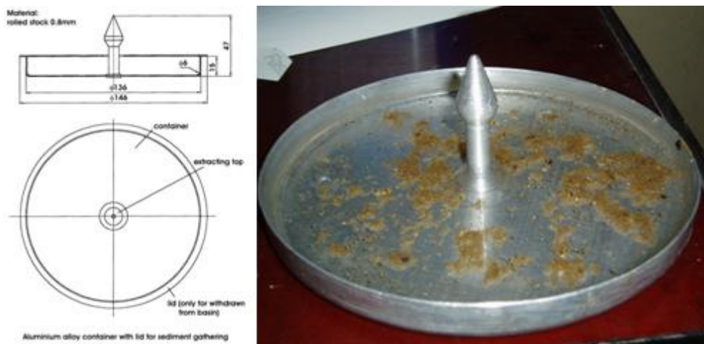
FIG. 14. Collector used in Romania. Made of Aluminium, with diameter equal to 20 cm (314 cm 2 ).
