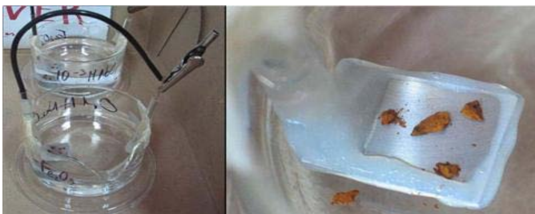
FIG. 23. Assembled galvanic couple in a cell (left). Sample detail, showing deposited oxide bits (right).
