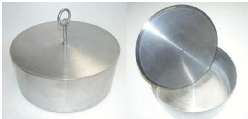
FIG. 12. Collector used at CCHEN, Chile. Material: AISI 304 stainless steel; dimensions: diameter 24.9 cm, height: 10 cm, Area: 486.9 cm 2 .
