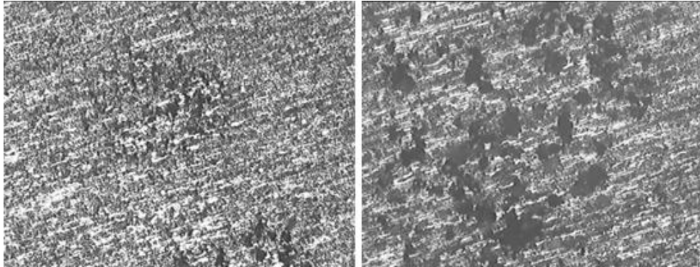
FIG. 26. Detail of surface under a deposit for a sample tested in 0.0001 N NaCl (FIG. 25). Left, region under deposit (200 \mu\text{m} ). Right, detail of pitting attack (points marked with "P") (100 \mu\text{m} ).
