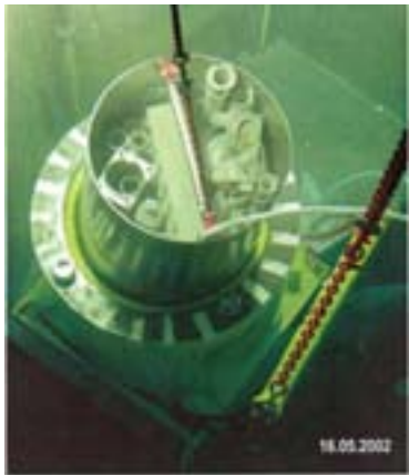
Fig. 1. Under-water loading of a GNS-Mosaik container.
