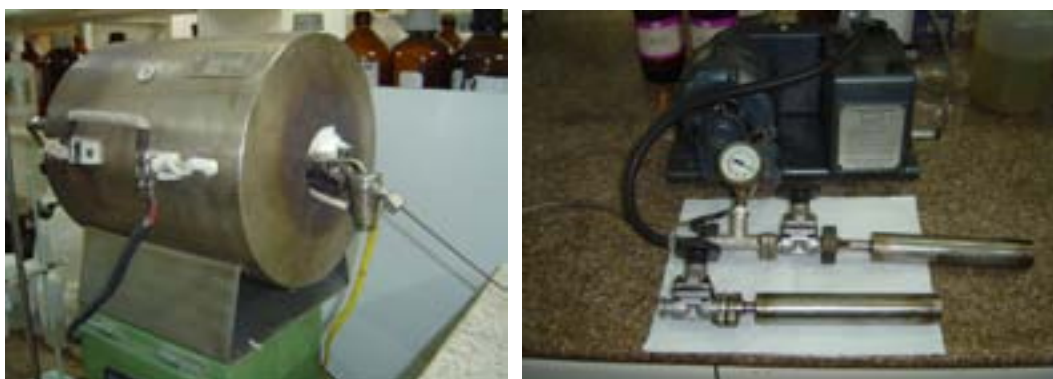
Fig. 3. Heating system (left) and vacuum pump with small steel cylinders (right).
