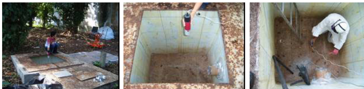
Fig. 11. Spectrometric measurements in the retention tank to identify the radionuclides.
