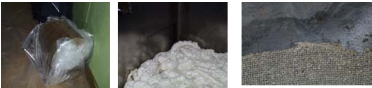
Figs. 19-21. Application of commercial polyethylene films, commercial polymeric foam and modified strippable coating for fixation or isolation of contaminations.
