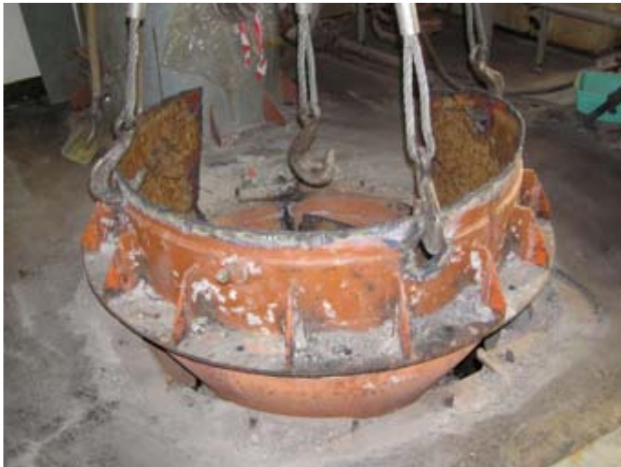
Fig. 10. Removing the separator after partial segmentation.
