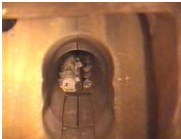
Fig. 3. Fuel element debris within FAZ fuel channel.
