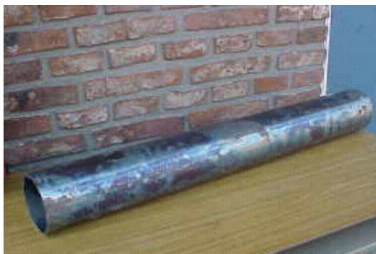
Fig 5: Upper part of Atucha 1 NPP coolant channel after oxidation process.
