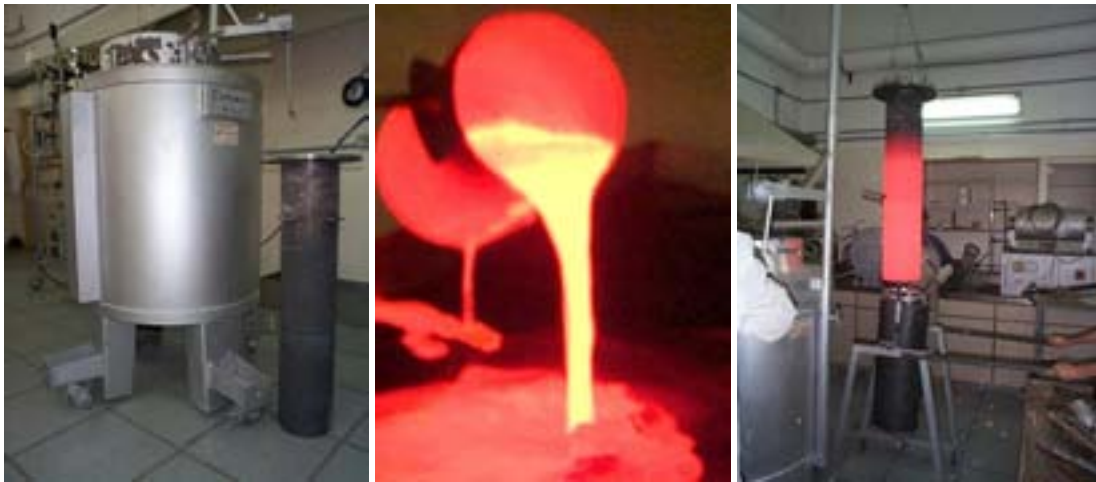
Fig. 7. Heating system and reactor (left), molten salt (center), reactor removal.
