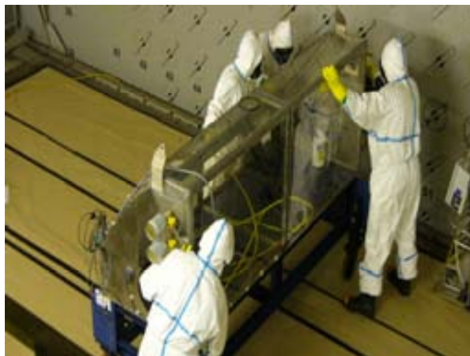
Fig. 8b. Interfacing the endoscope with Pile 1 charge face inspection in Pile 1.
