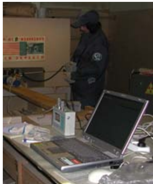
Fig. 10 Radiological survey with application of gamma-, beta- spectrometers and dosimeters in the case of unknown radionuclide composition.
