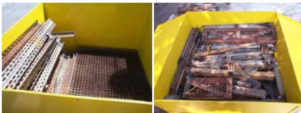
Fig.25. Contaminated structural parts of carbon steel stored in steel boxes.
