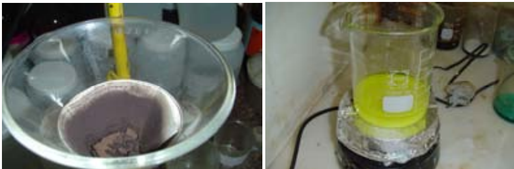
Fig. 8. Filtering to separate the oxides present in the salt and salt crystallization.
