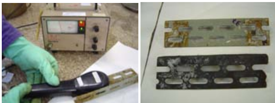
Fig. 29. Monitoring (left), items before (above right) and after stripping (bellow right).
