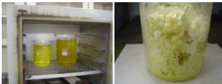
Fig.31. Crystallization of the filtrate by heating (left) and recovered salt (right).
