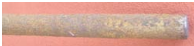
Fig. 7: External appearance of carbon steel bars after oxidizing process.
