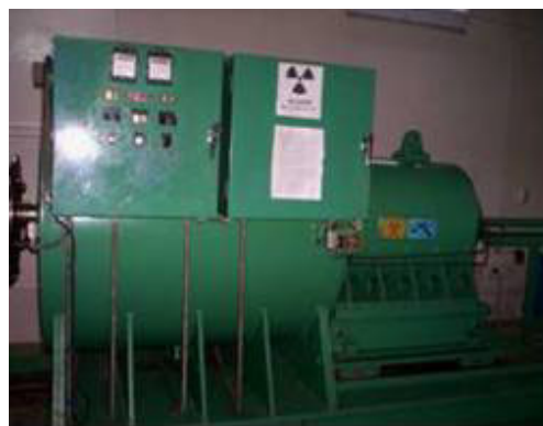
Fig. 7. Irradiator facility Gammacell 500, source storage container (the smaller cylinder).
