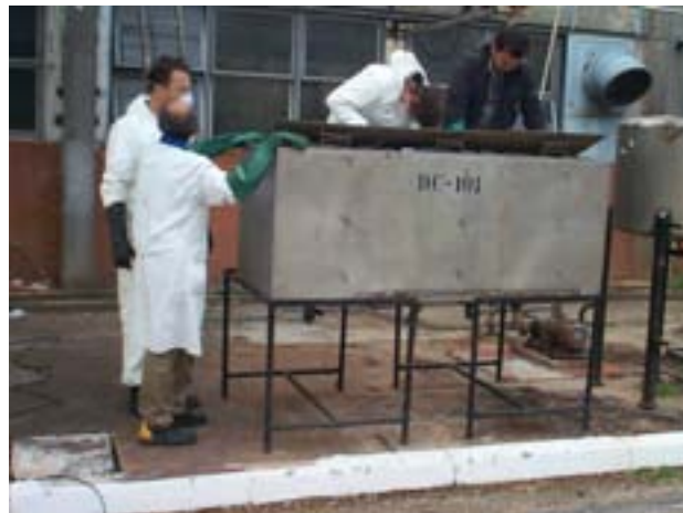
Fig.21. Stainless steel tank adapted for decontamination of components.
