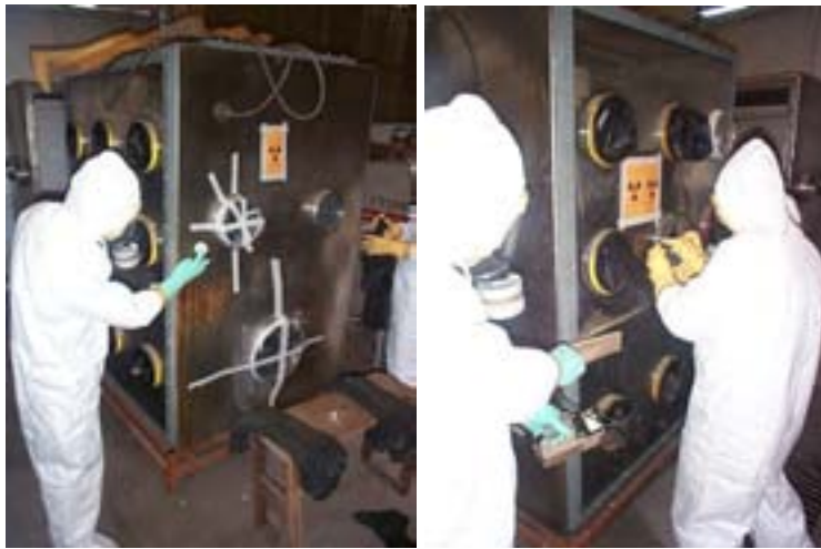
Fig. 13. A larger glove-box, previously used in the process (already contaminated) is being prepared for future assembling of the molten salt equipment.
