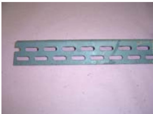
Fig.26. Painted carbon steel submitted to acid pickling (left side) with small effect.
