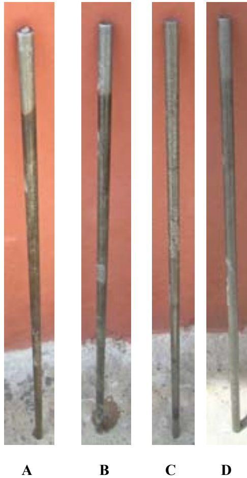
Fig 8: Evolution of the cleaning process for A: 6 minutes, B:15 minutes, C: 30 minutes and D:60 minutes.
