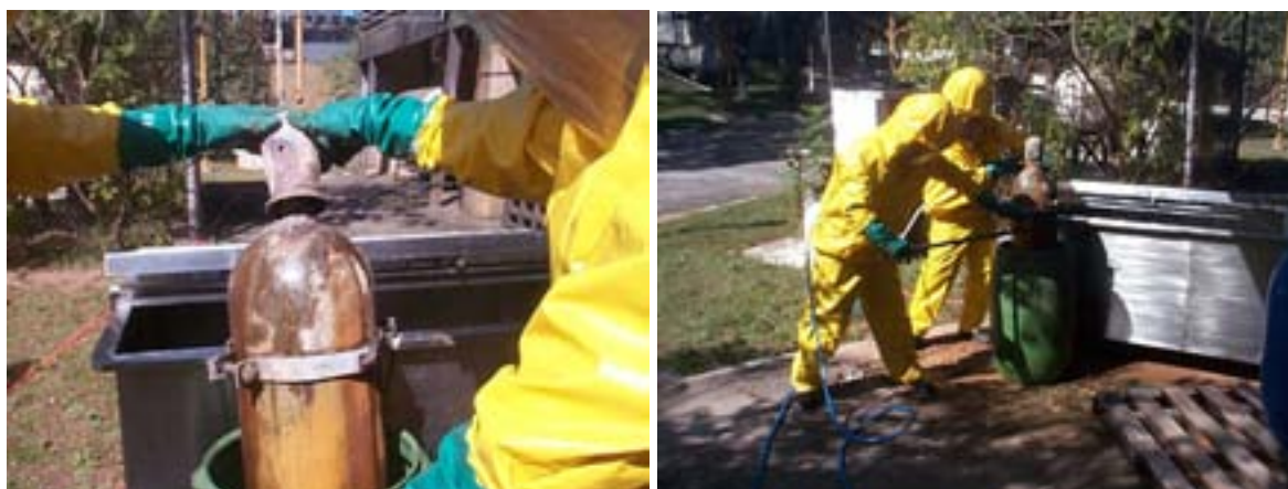
Fig. 2. HF cylinder emptying operation and neutralizing of the acid solution.
