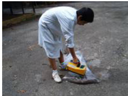
Fig. 21. Monitoring of materials removed from the retention tank.
