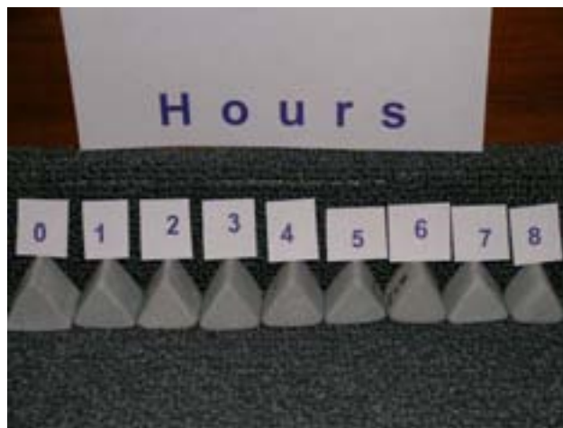
Fig. 17d: Abrasive media samples from 0 until 8 working hours.
