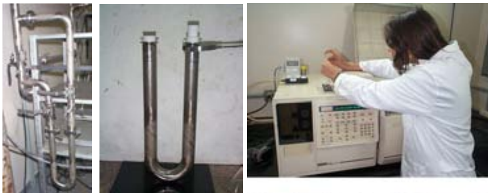
Fig.17. Gas sampler and CG/MS analysis.
