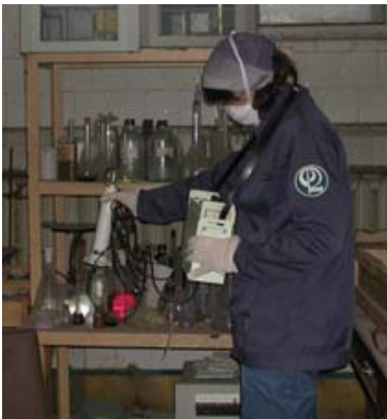
Fig. 9 Radiological survey in old radiochemical laboratory with known radionuclide composition.
