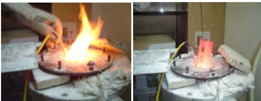
Fig. 27. Molten salt stripping - introduction (left) and removal (right) of the sample.
