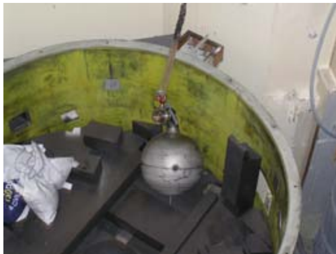
Fig. 12 The core vessel lifted out.
