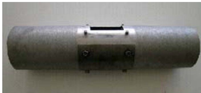
Fig 9: Frontal and internal view of the device used to test ability for cleaning internal areas.
