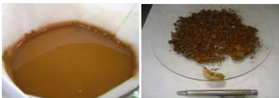
Fig.30. Filtration of the solution obtained from the salt and the final solid waste.
