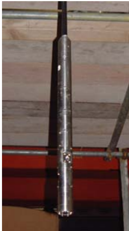
Fig. 6. Intrusive inspection equipment for foil hole examination in Pile 1.
