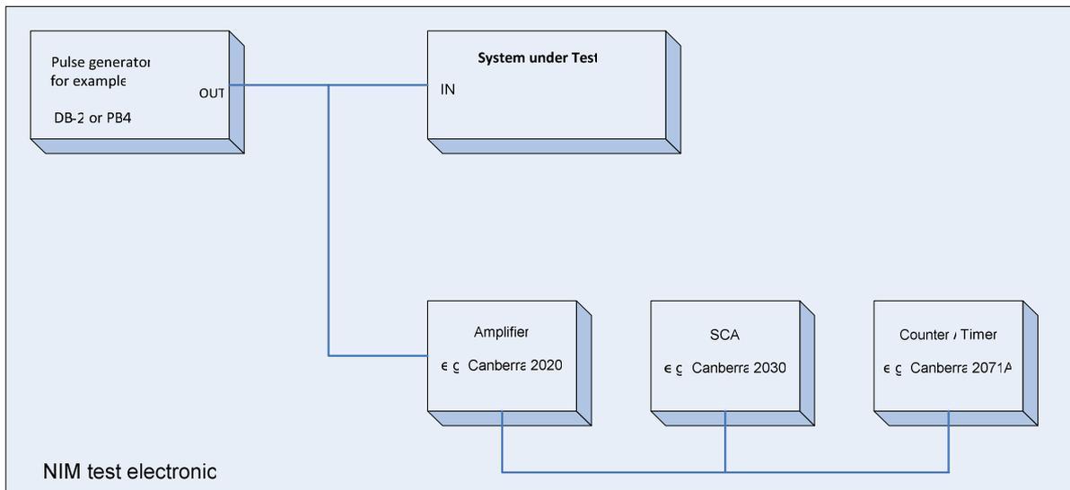
Fig. 3. Set up for integral non-linearity measurements.
