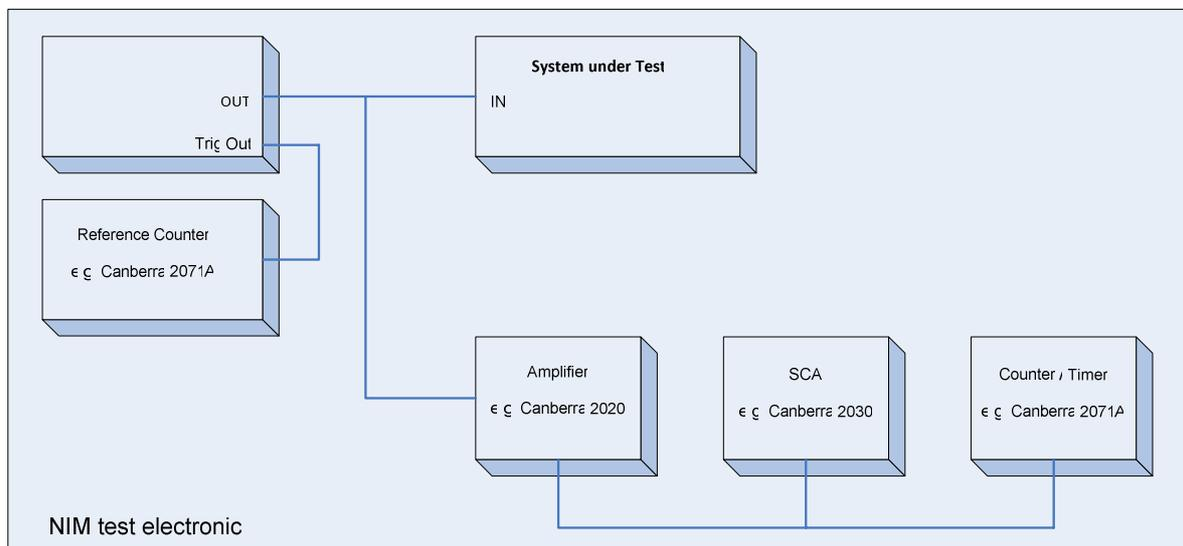
Fig. 2. Test set up for clock accuracy measurements.
