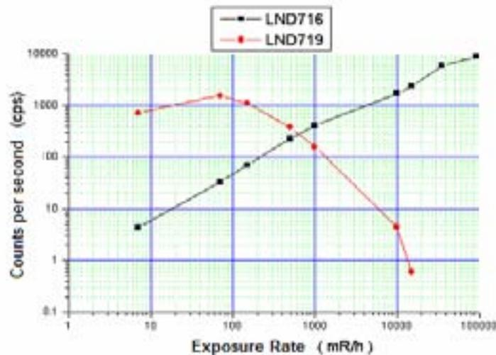
Fig. 8. Comparison between the responses of a GM detector specially designed for high exposure rates (LND716) and a normal detector (LND 719).
