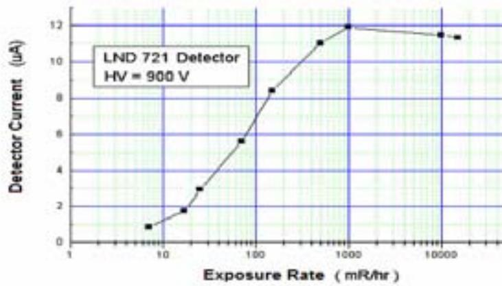
Fig. 7. Increment of the current in the GM detector due to the increase of the exposure rate.
