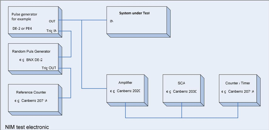
Fig. 5. Test set up for count rate non-linearity measurements.
