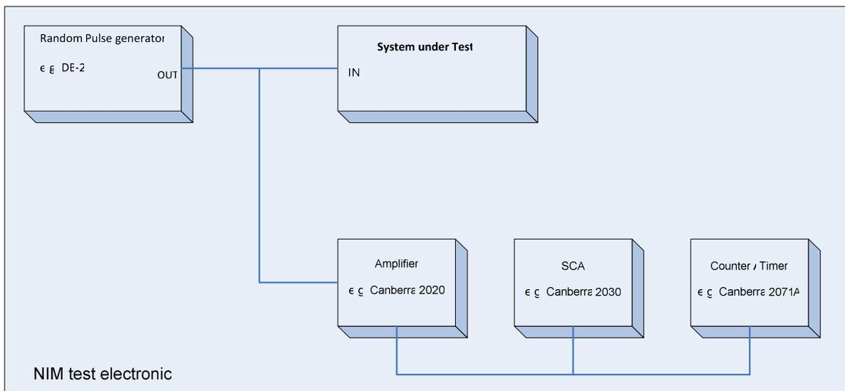
*Fig. 6. Set up for peak shift versus count rate measurement.*
