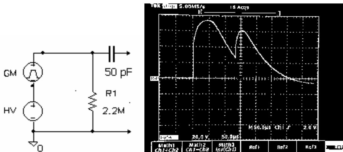
Fig. 1. Dead time measurement. a) (Left) Biasing circuit; b) (Right) Pulses obtained for the LND 721 detector, the settings of the oscilloscope are: 20 V/div and 50  $\mu$ s/div.
