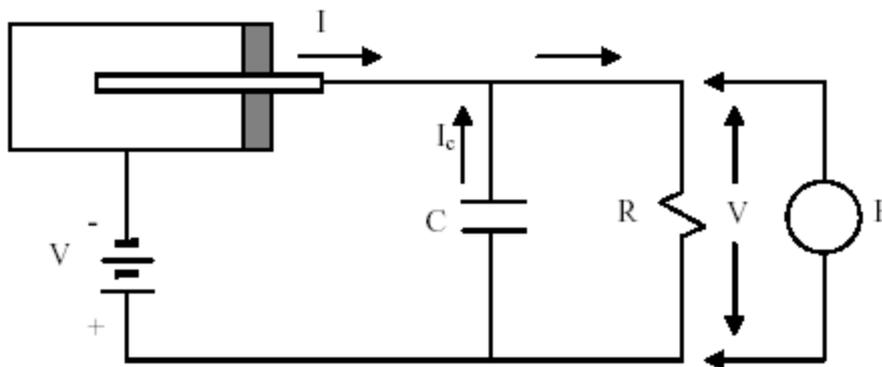
Fig. 3. Ionization current measurement (charge method).
