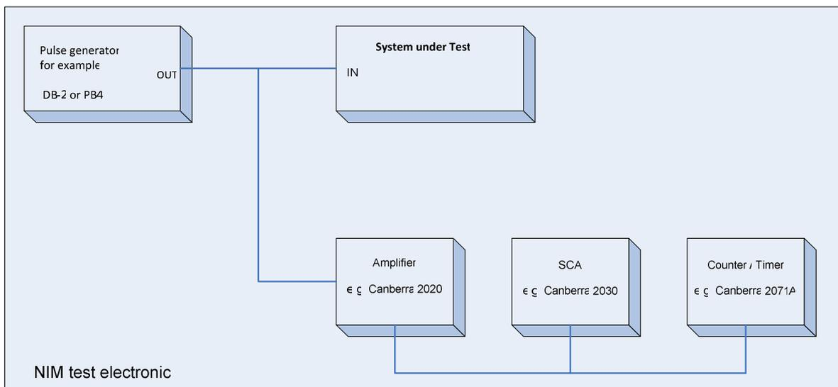
*Fig. 1. Test set up for count accuracy determination.*
