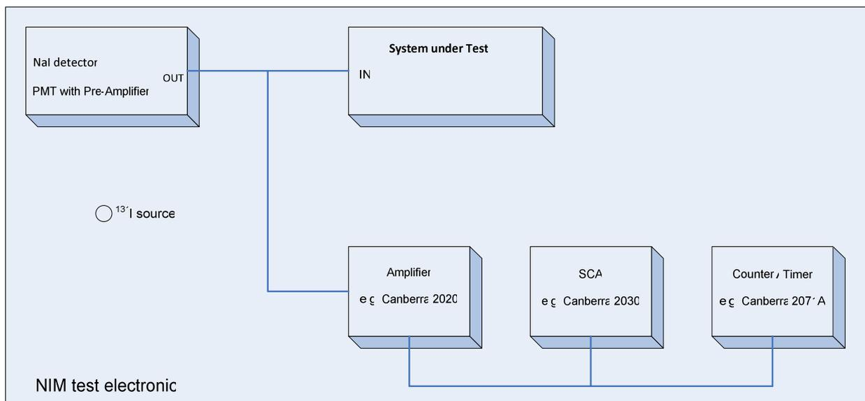
Fig. 7. Set up for chi square test.
