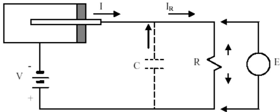
Fig. 2. Ionization current measurement (electrometric method).
