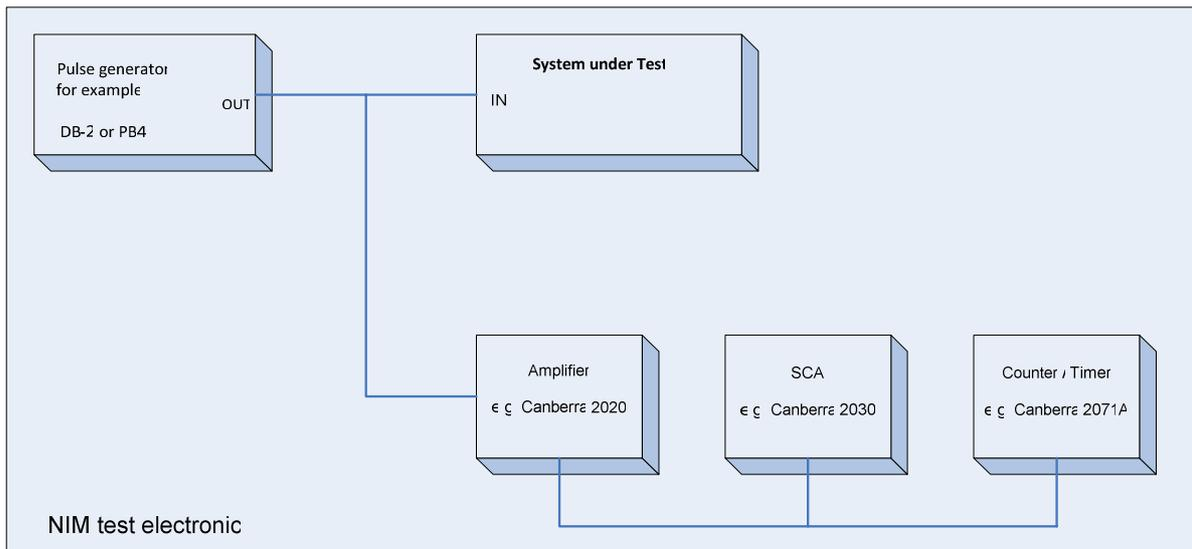
Fig. 4. Set up for differential non linearity measurements.
