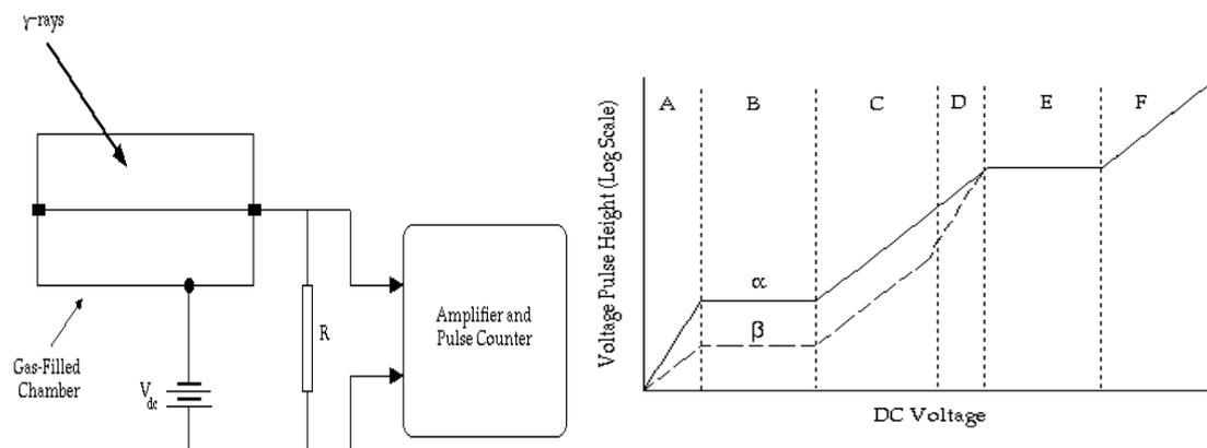
Fig. 1. Gas filled detectors and counting plateau.
