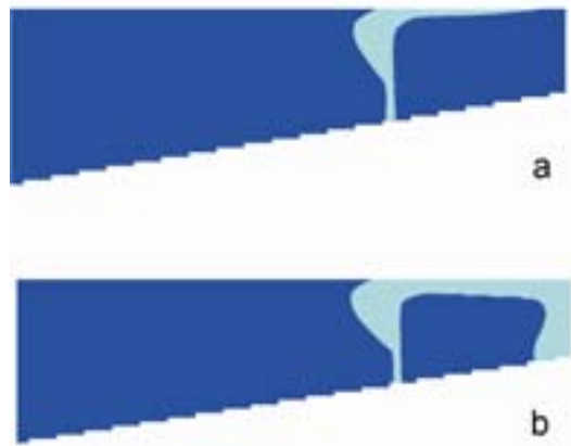
FIG.4. Salinity distribution in the vertical section of Bay A, simulation by PCFLOW3D model. (a) T = 2h\ 00\ min ; (b) T = 2h\ 15\ min .
