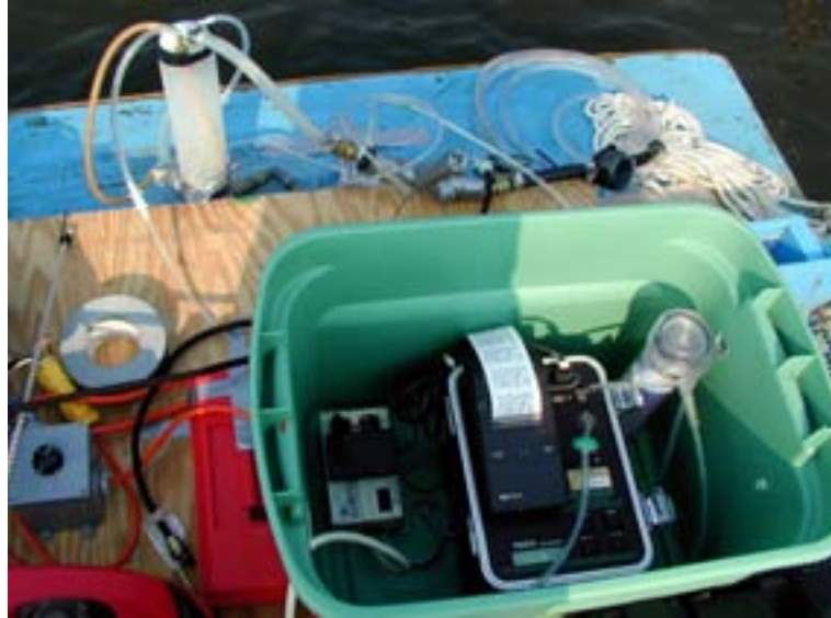
FIG.1. Photo of the water exchanger – RAD-7 continuous monitoring system.
