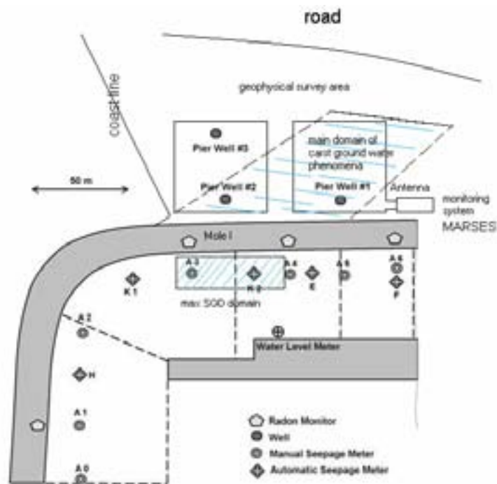
FIG.4. Geophysical survey area and locations of manual and automated seepage meters.
