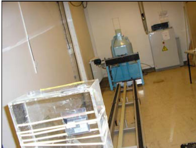
Figure 5.7 Irradiator containing two photon sources ( ^{137}\text{Cs} and ^{60}\text{Co} ).
