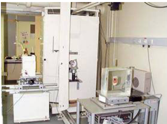
Figure 5.5 X ray generator ISOVOLT HS 320 kV (SEIFERT) used for N-80 and N-120 beam qualities.
