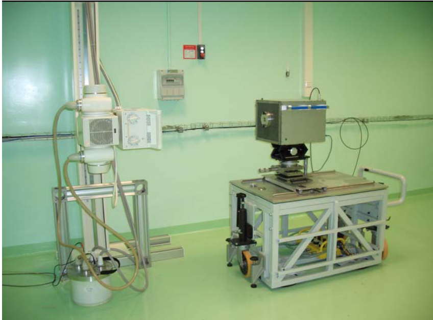
Figure 5.8 Diagnostic X ray facility, on the right hand side the specially designed free air chamber used for measuring the air kerma.
