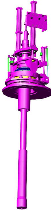
*FIG. 11. Example of a transferred torch.*
