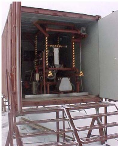
*FIG. 9. Mobile test facility for thermochemical treatment of ion exchange resins.*
