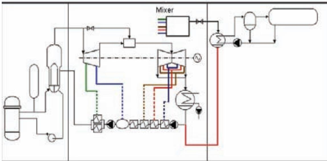
Figure 27. Coupling scheme with mixing the flow rates from the various internal bleed-off points
