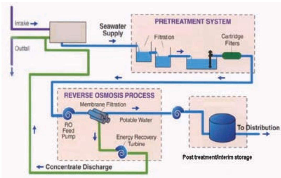
Figure 23. Schematic illustration of an operating RO plant.
