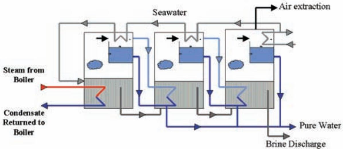
Figure 21. Schematic diagram of an MED system.
