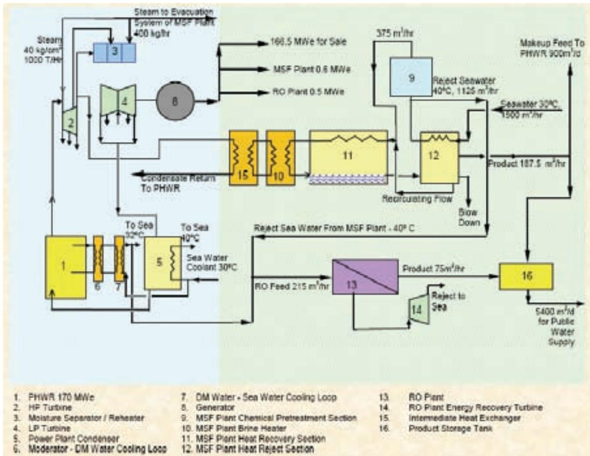
Figure 36. Hybrid MSF-RO coupling to the PHWR at Kalpakkam (India).
