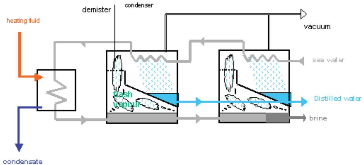
Figure 20. Schematic diagram of an industrial MSF design.
