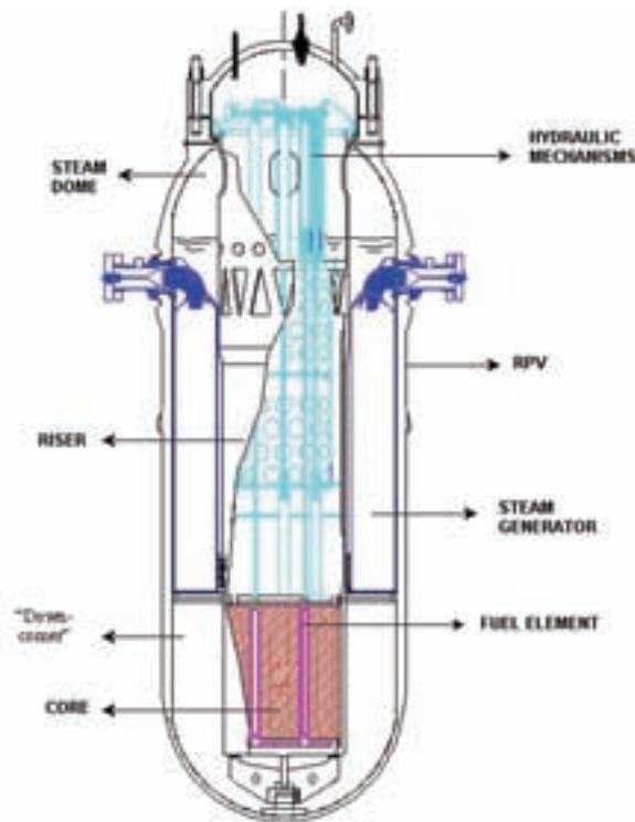
Figure 3. General view of CAREM reactor assembly.
