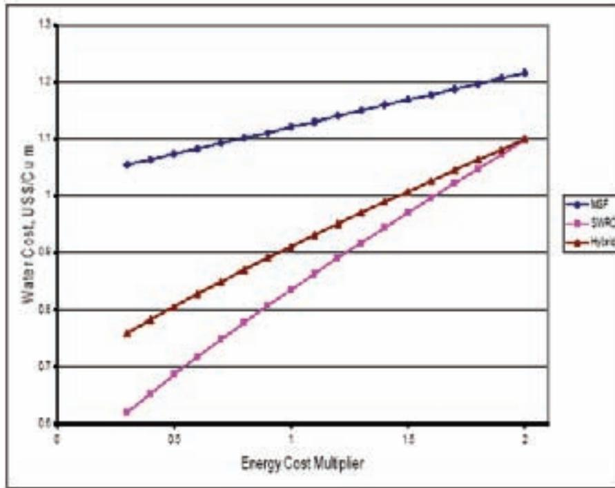
Figure 37. Variation of hybrid, RO and MSF water costs with the power cost.
