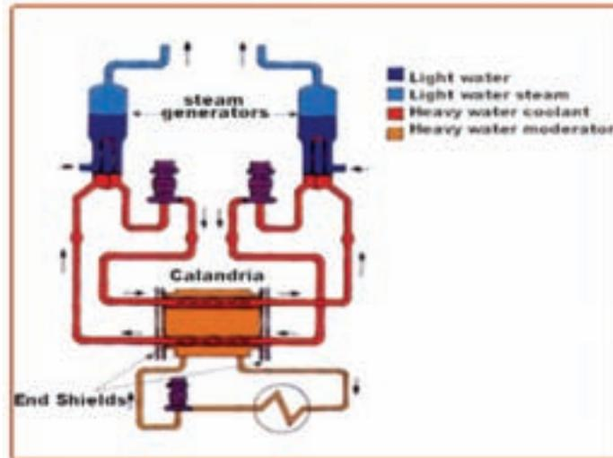
Figure 12. Simplified flow diagram of the MAPS PHWR at Kalpakkam.
