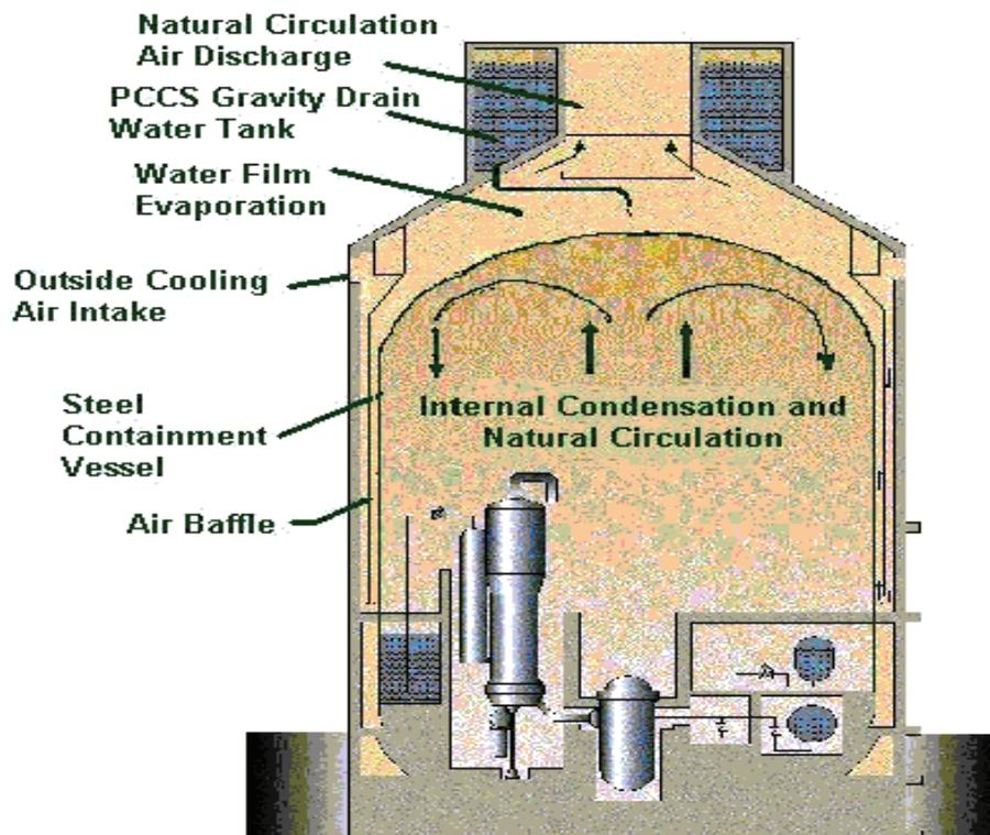
Figure 5. Schematic layout of the AP-600 nuclear island.
