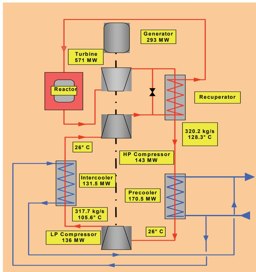
Figure 8. GT-MHR flow diagram.
