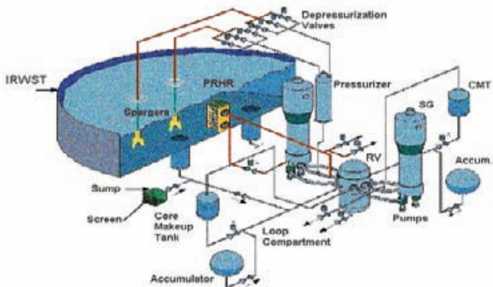
Figure 6. AP-600 Passive Containment Cooling System (PCCS).
