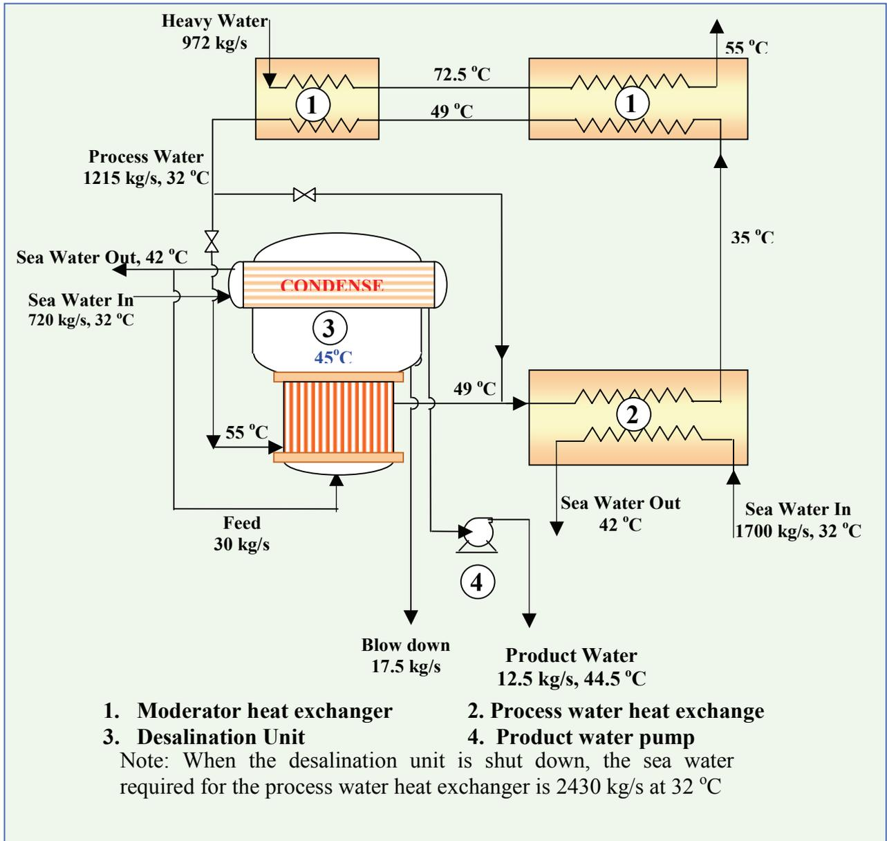
Figure 35. PHWR500 coupling scheme, utilising waste heat.
