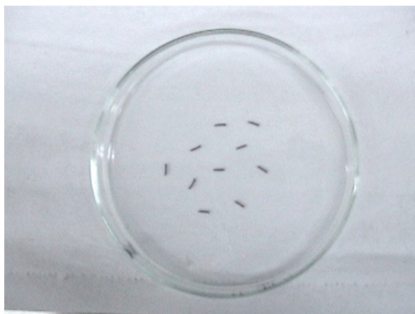
FIG. 4. Silver wires coated with palladium employing the Simple Method
