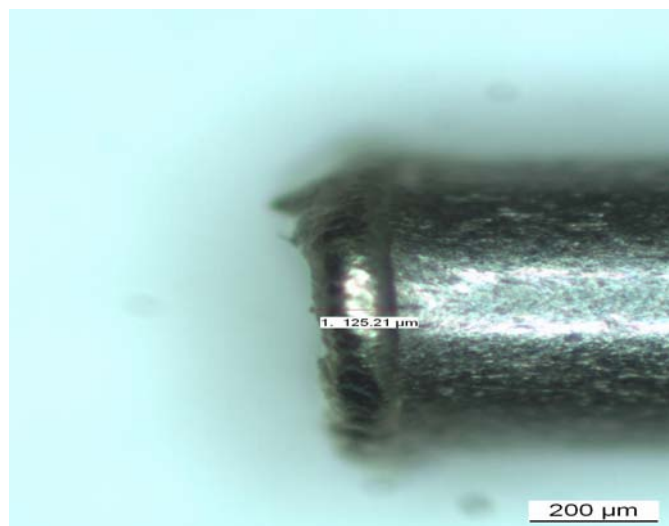
FIG. 12. Laser welding of titanium tube with 0.05 mm Ti cap.
