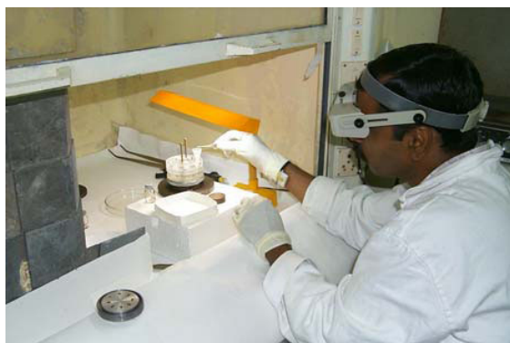
FIG. 4. Loading of ^{125}\text{I} source core inside the capsules
