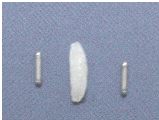
FIG. 2. The sizes of these sources are like a grain of rice (0.8 mm OD x 4.5 mm long)
