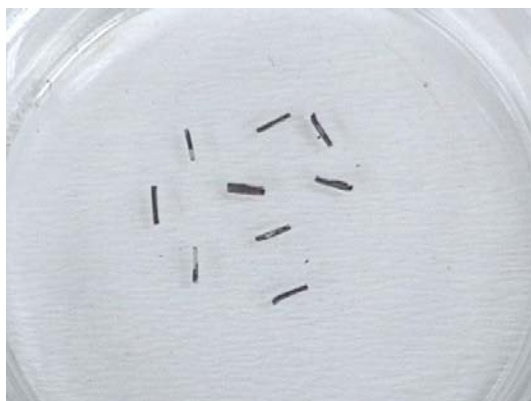
FIG. 5. Silver wires coated with palladium employing the Complex method
