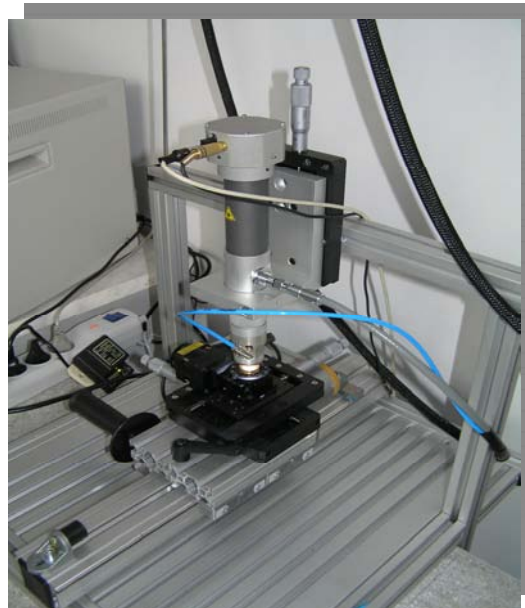
FIG. 7. Positioning of welded element against the laser beam
