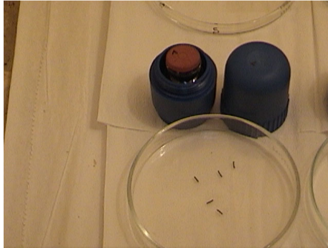
FIG. 8. Group G9 of silver wires coated with palladium after the process of adsorption of ^{131}\text{I} during 6 hours
