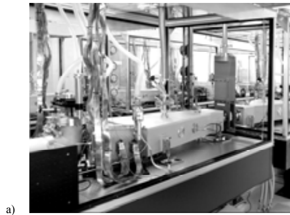
Figure 1. A picture of the Mercury laboratory showing dual amplifiers and Class 1000 clean room enclosures which minimize air turbulence and decrease optical damage due to contaminants.
