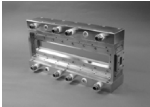
Figure 2. Laser head without LD modules.
