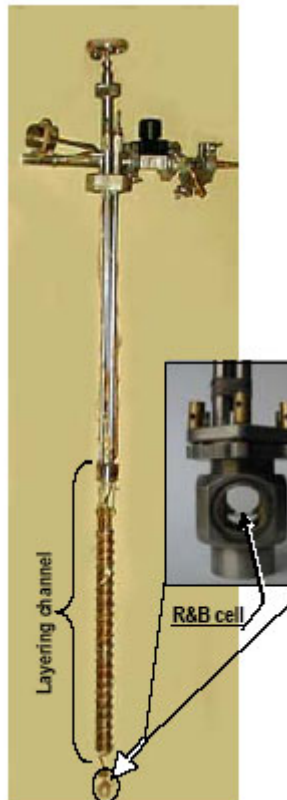
Figure 3. In the R&B cell layer symmetrization & freezing take place within the same small area.
