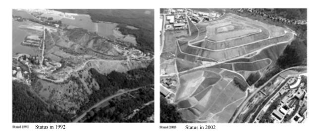
FIG. 3. Illustration of the in situ remediation of the waste rock dump 366 in the vicinity of Schlema.
