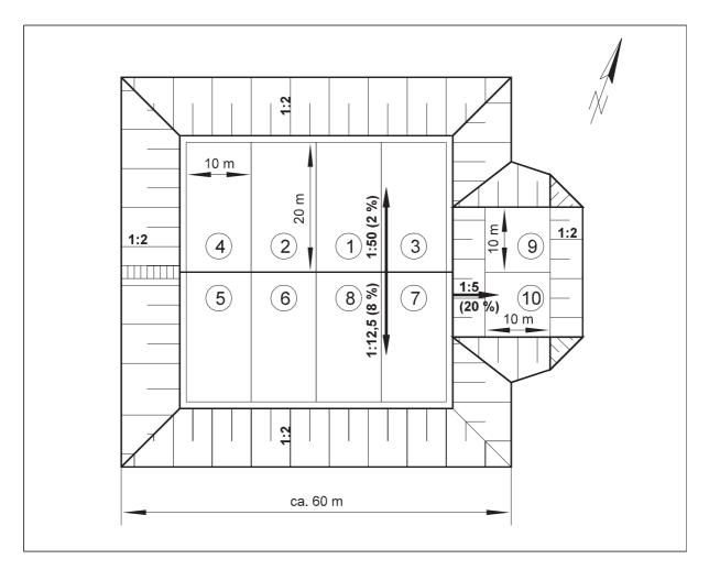
FIG. 4. Map of the final cover test field site.
