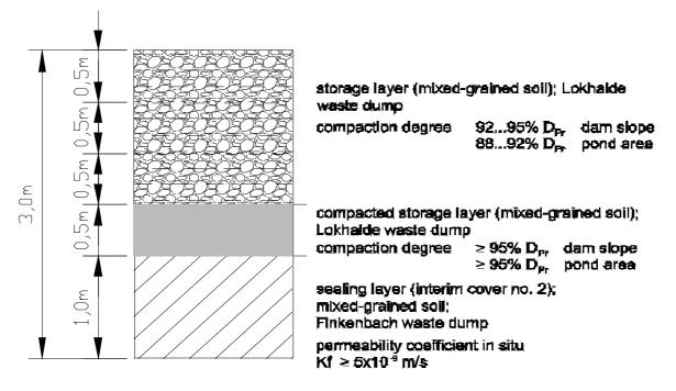
FIG. 5. Layering of the final cover on the northern tailings beaches of Pond A.
