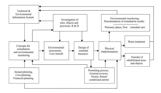
FIG. 1. Remediation workflow at WISMUT
