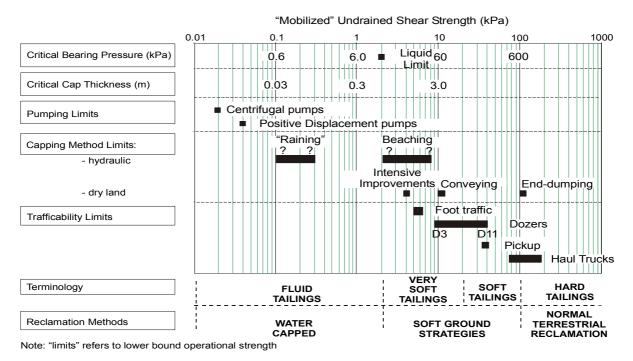
FIG. 4. Remediation methods as a function of tailings shear strength and critical parameters.
