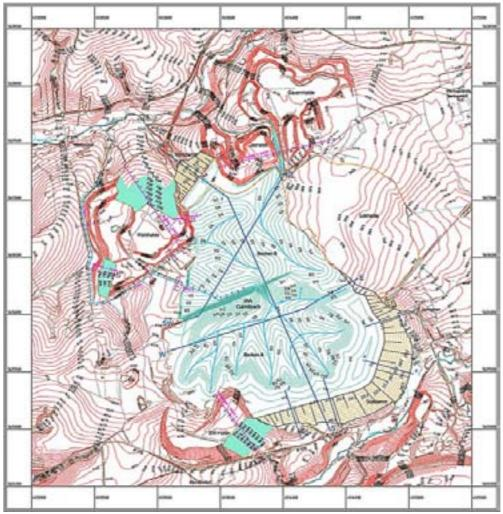
FIG. 3. Conceputal design of the re-contoured Culmitzsch tailings pond.
