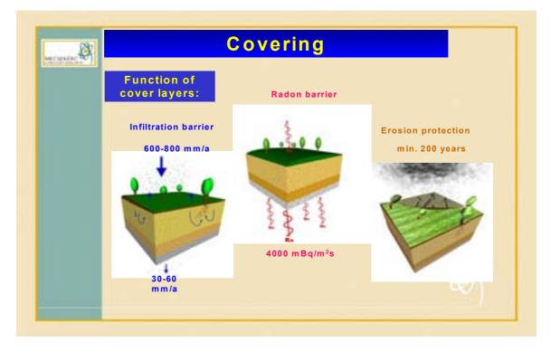
FIG. 3. Function of the covering layer.
