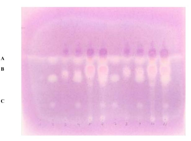
FIG. 5. LOD with cow liver extract enzyme inhibition and  $\beta$ -naphthyl-acetate substrate (E $\beta$ NA) after GPC cleanup.
