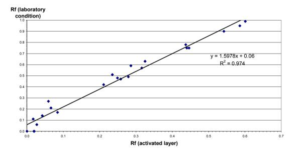
FIG. 3. Comparison of Rf of pesticides on freshly activated layer and on equilibrated one to room conditions. Eluent: petroleum ether + diethylether = 1+2.
