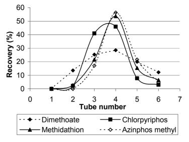
FIG. 1. Calibration of GPC system.
