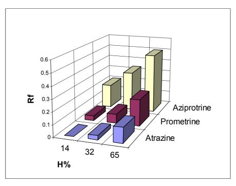
FIG. 4. Effect of relative humidity (H%) on HRf.c b.
