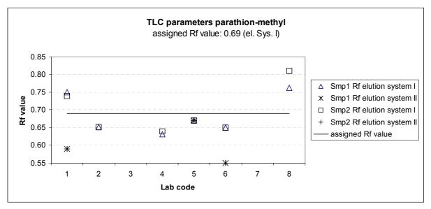
FIG. 4. Results of inter-laboratory comparison test with parathion-methyl.
