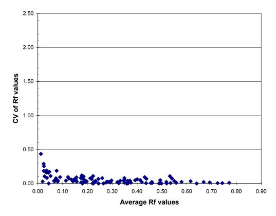
FIG. 6. The coefficient of variation, CV, of Rf values as the function of Rf values in elution System VI.
