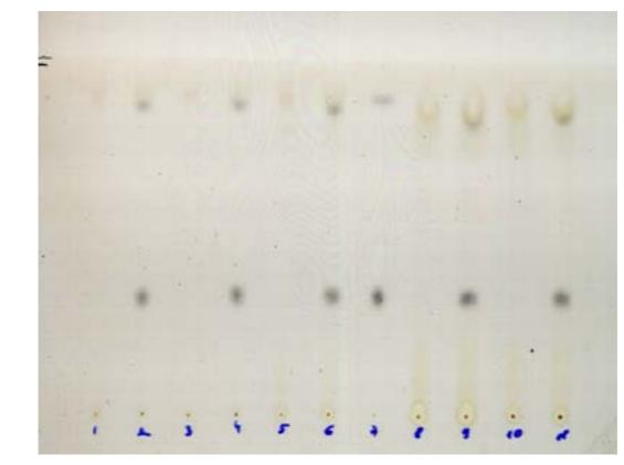
FIG. 7. LOD with silver nitrate (AgUV) reaction after GPC cleanup.
