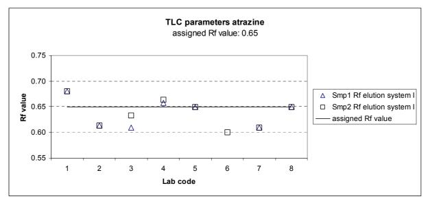
FIG. 3. Results of inter-laboratory comparison test with atrazine.
