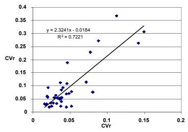
FIG. 9. Relation of between-laboratories  $CV_R$  and within-laboratory CVr of Rfs values.
