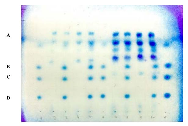
FIG. 6. LOD with pig blood serum enzyme inhibition and acethylthiocholine iodide substrat (EAcI pig) after GPC cleanup.
