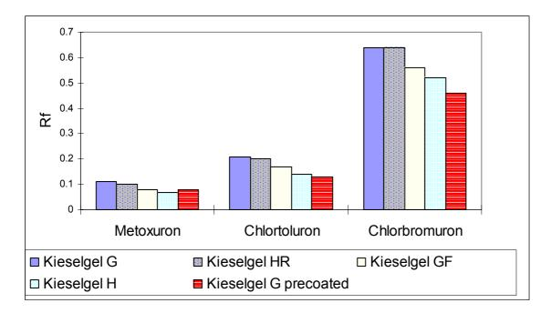
FIG. 1. Effect of the type of silica on Rf with eluent n-hexane+diethylether = 1+2.
