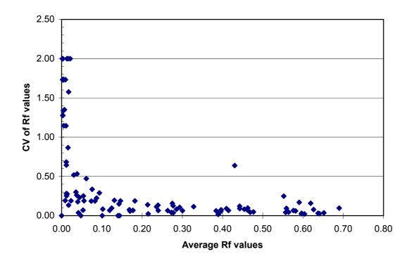
FIG. 3. The coefficient of variation, CV, of Rf values as the function of Rf values in elution System III.
