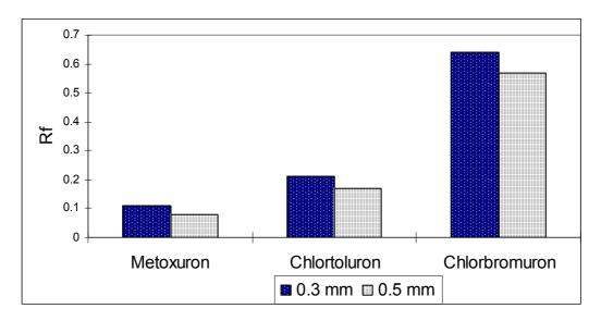
FIG. 2. Effect of thickness of silica-layer on the HRf with eluent n-hexane + diethylether = 1+2.
