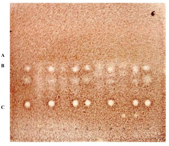
FIG. 4. LOD with fungi spore inhibition (FAN) after GPC cleanup.
