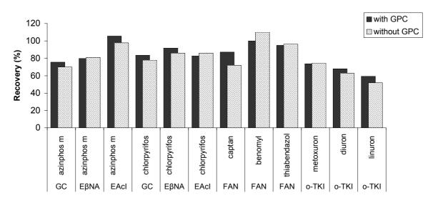
FIG. 2. Recoveries obtained by different quantification methods with and without cleanup.
