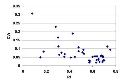
FIG. 11. Relation of between-laboratories  $CV_R$  of Rf values and the Rf.
