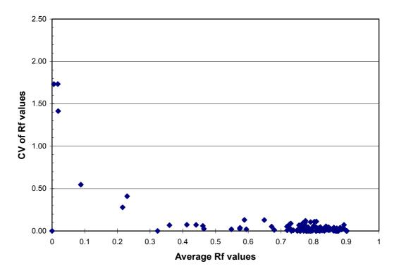
FIG. 5. The coefficient of variation, CV, of Rf values as the function of Rf values in elution System V.
