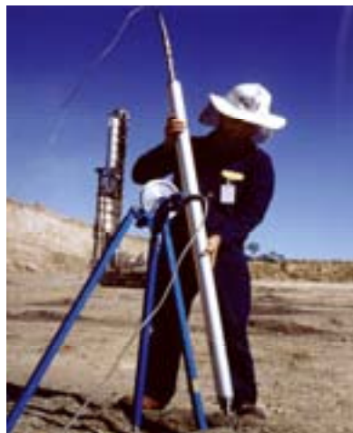
FIG. 18. Low radiation intensity (1.1 MBq) gamma spectrometric borehole logging probe for coal delineation and coal raw ash content.
