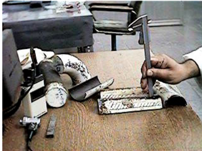
FIG. 11. Mechanical measurements on the corroded pipe sample TUR-FAB-P3 which is destructed.
