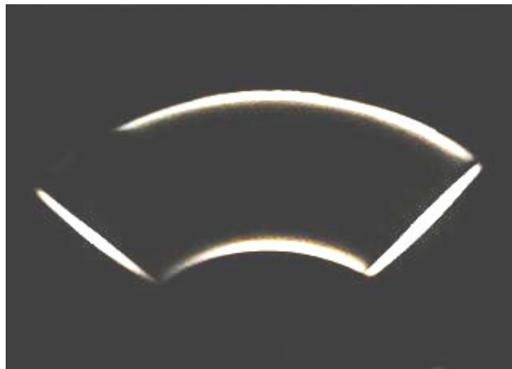
FIG. 7. Print of radiograph of sample TUR-FAB-E2 (exp. pos1, SFD: 700 mm, 200 kV, 5 mA, 5 min, Film: Agfa D7 Pb, Density: 4).
