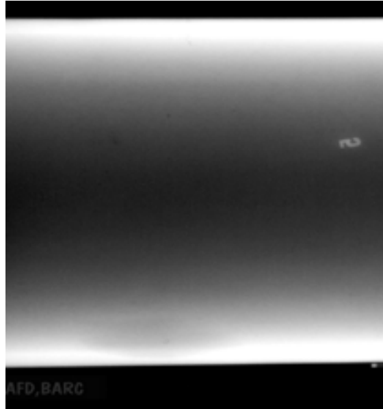
FIG. 7. Digital radiograph of pipe MAL-FAB-3 showing notch at edge.
