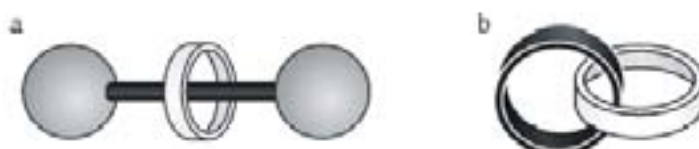
FIG. 1. Schematic representation of a rotaxane (a) and a catenane (b).
