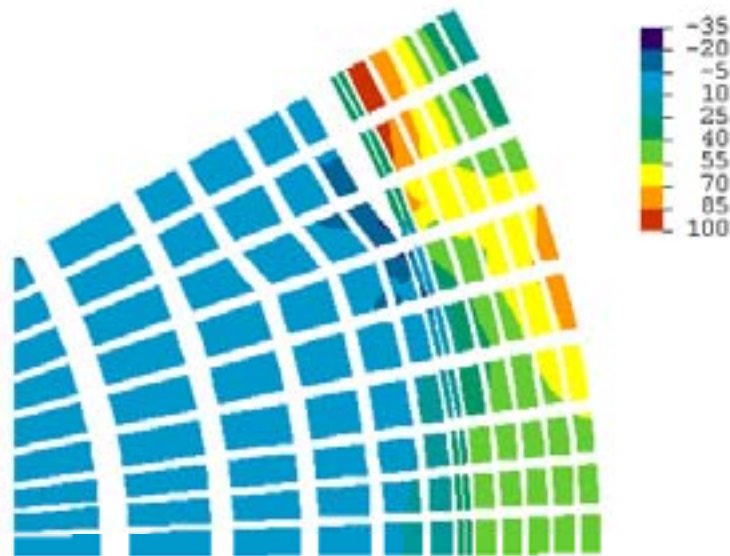
FIG. 15. Hoop Stress Contour Results for Rod B4.
