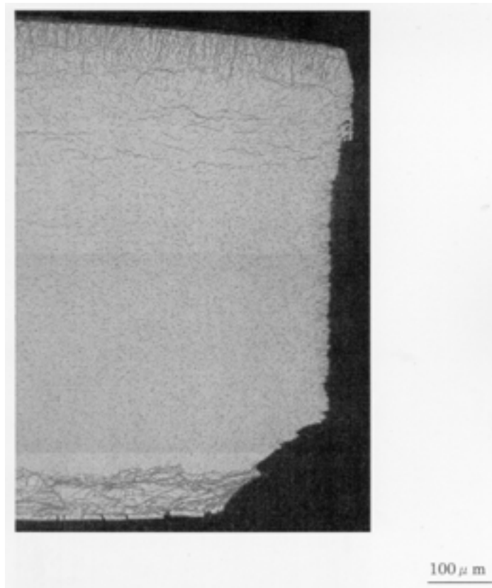
Photo 6. Hydride Distribution in Cladding of Failed Segment Rod.
