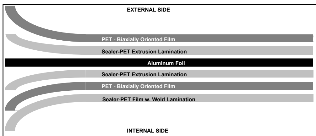
FIG 1. Suggested laminate ensemble for high-dose radiation-sterilised food-packaging.
