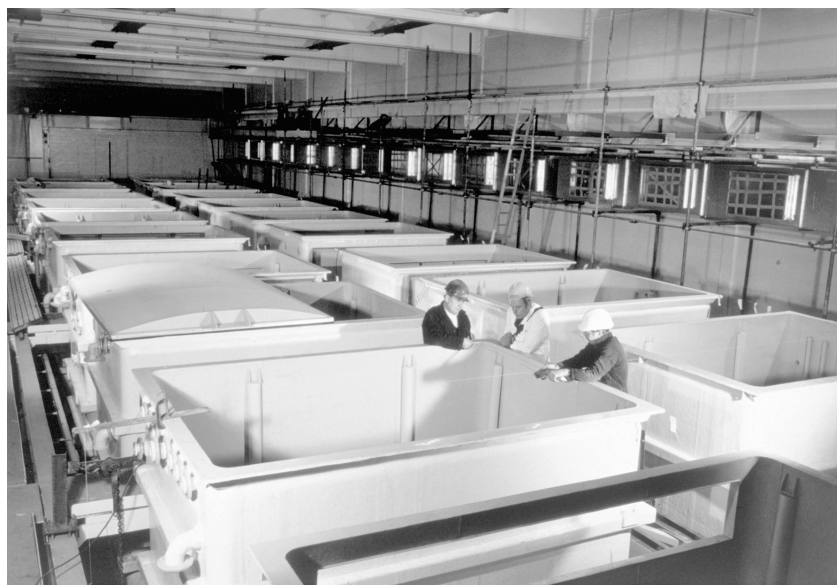
FIG. 16. Plant for large scale chemical decontamination operation.
