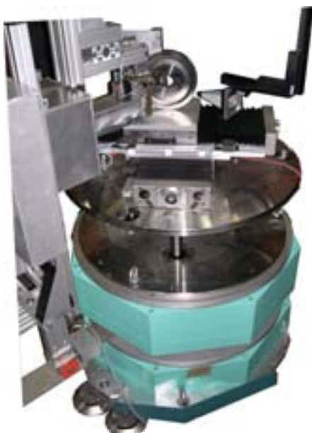
Figure 2. An X-Y-Z translation device is mounted on a HUBER sample table to move the sample (here: MTU turbine wheel) through the gauge volume defined by the slit system.
