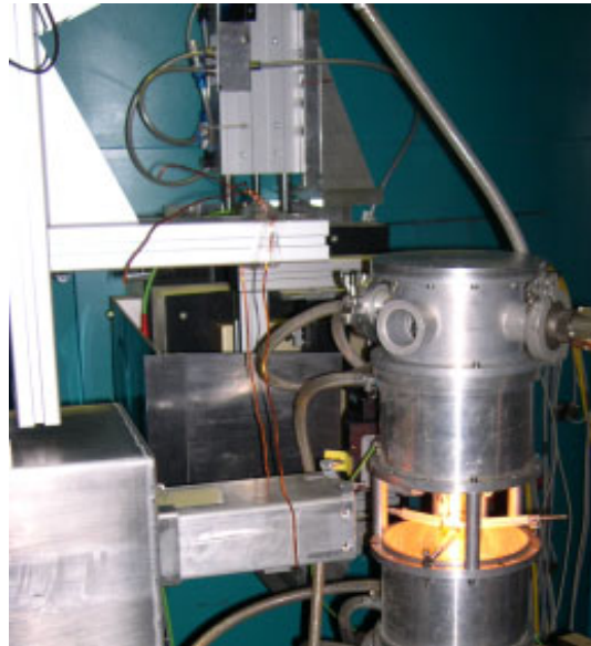
Figure 10. The high temperature furnace mounted on the sample table of E7.
