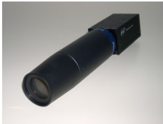
Figure 6. A high resolution camera (JAI M4+) together with telecentric optics (JENMETA 1:1) allows very accurate sample positioning on the sample table.
