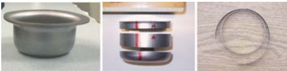
Figure 11. Standard test specimen for the measurement of springback stresses. Left: intact cup; middle: sectioned cup with mid-section as the actual specimen; right: split mid-ring for measuring the ring opening.
