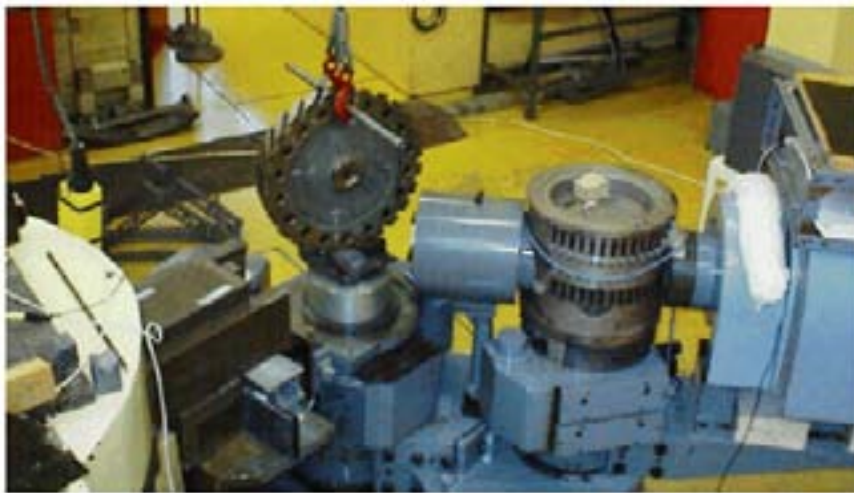
Figure 6. The material NiCrMoV high-strength-low-alloy steel with reference to the ASTM A 471 (type 2) The wheel experimented, as bladed, \sim 2500 0-peak cycles, with some 102% over speed ones, and operated at a temperature \sim 300 °C.
