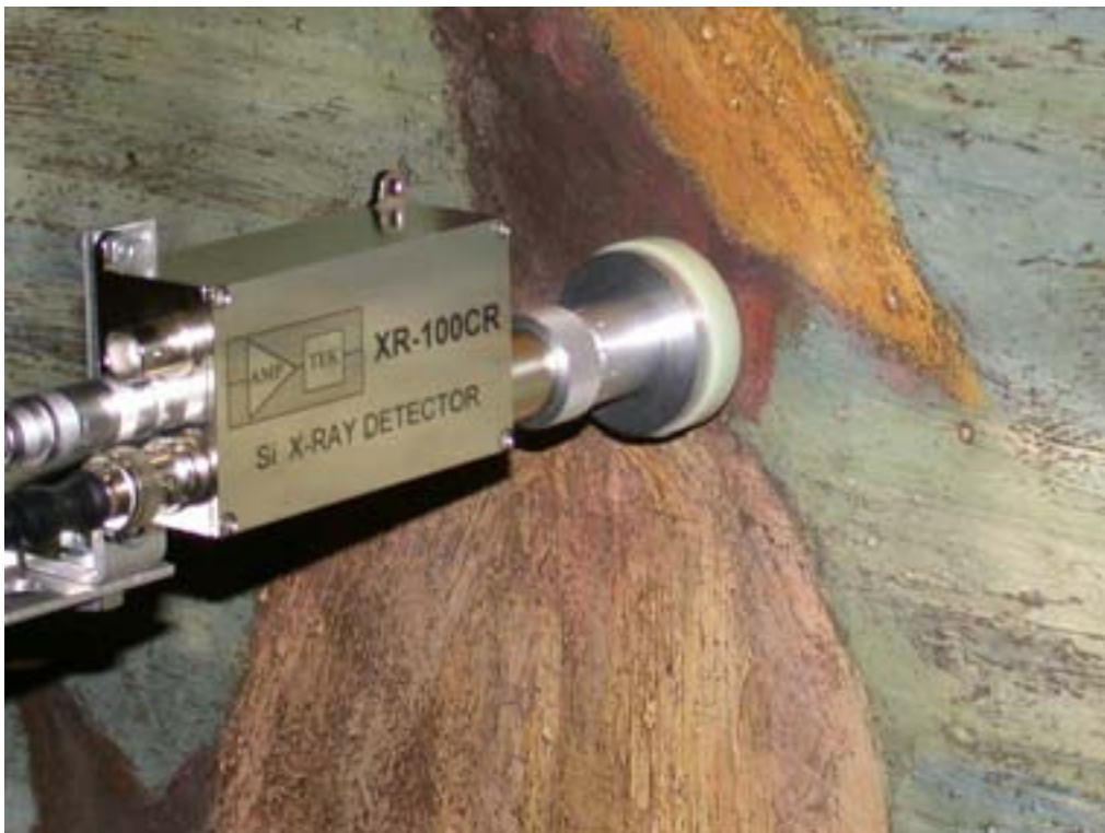
Fig. 5. The AMPTEK XR-100CR detector equipped with the ^{109}\text{Cd} excitation head.
