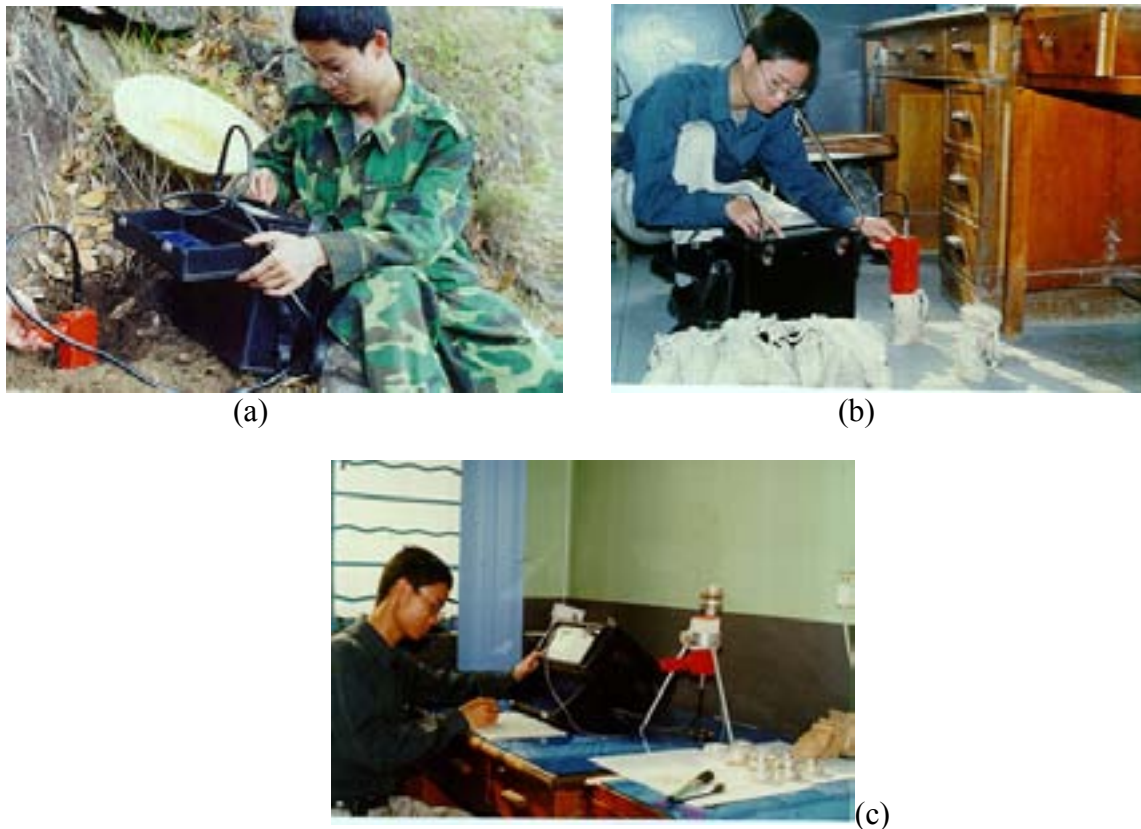
Fig. 7.2. In situ FPXRF measurement with the IED2000P FPXRF analyser. (a) Analysing natural soil in a shallow hole in the field. (b) Analysing a natural soil sample in the tent. (c) Analysing a powdered sample in the field station.
