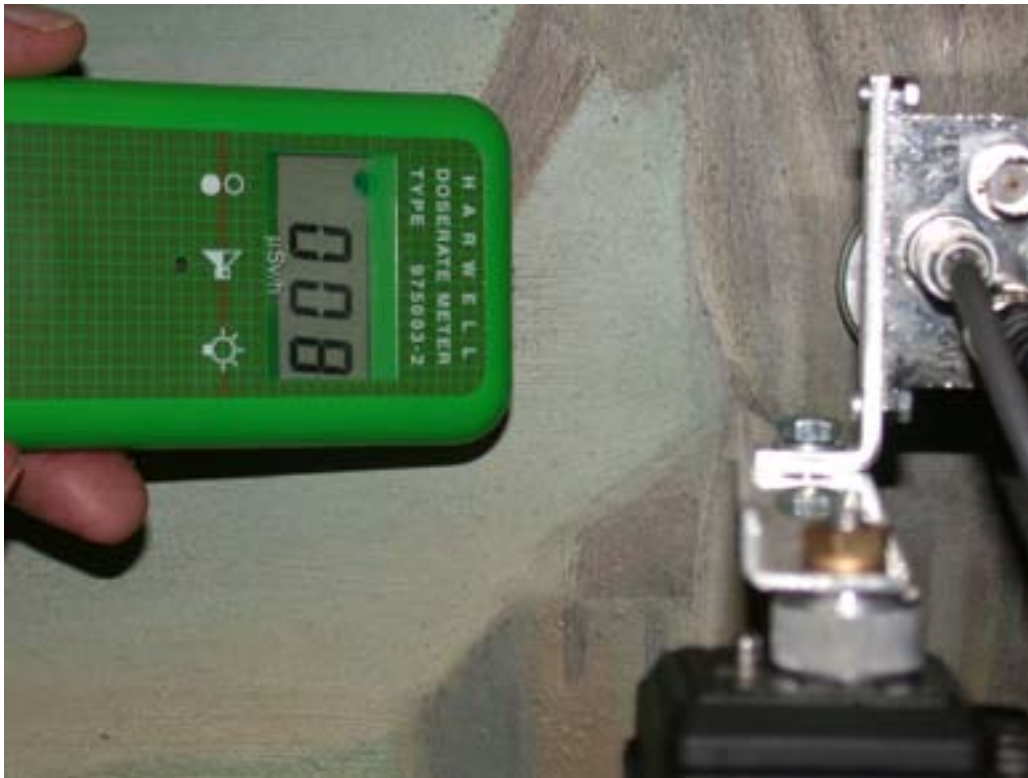
Fig. 21. Control of the dose caused by the portable XRF excitation head around the analysed spot.
