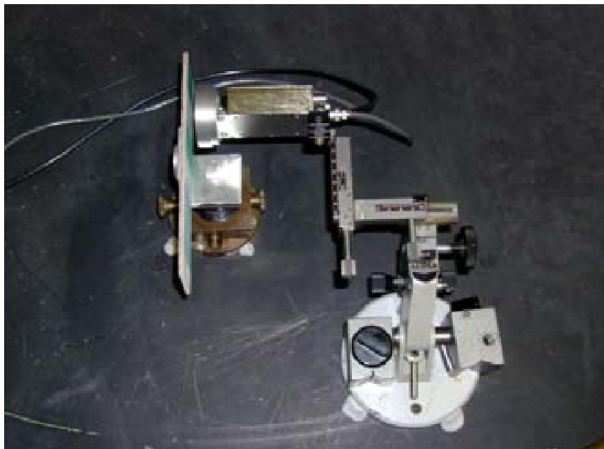
Fig. 2. Top view of the XRF setup with the AMPTEK XR100T detector holding the NEN ring source in an Al housing.
