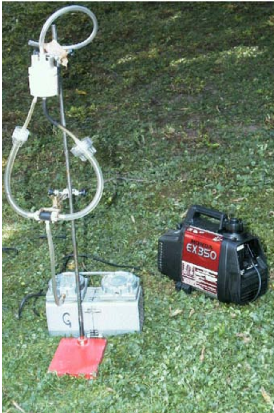
Fig. 11. Aerosol sampling by a dichotomous sampler.
