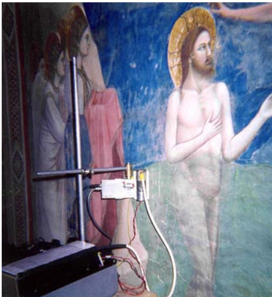
Fig. 2. Equipment for analysis of elements from 1 to 30 keV employed in the Chapel of the Scrovegni in Padua, composed of a W-anode 30 kV, 0.3 mA X ray tube and a thermoelectrically cooled Si-PIN detector.
