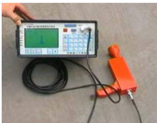
Fig. 7.1. The IED-2000P FPXRF analyser made by our research group.
