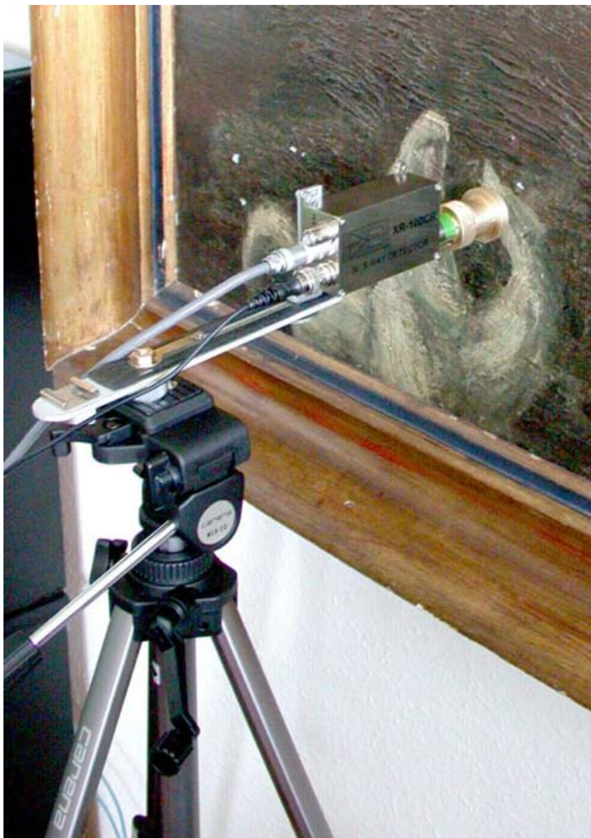
Fig. 12. The portable XRF setup composed of an AMPTEK X ray detector equipped with an excitation head containing the ^{55}\text{Fe} ring source in front of the debated Csontváry painting.
