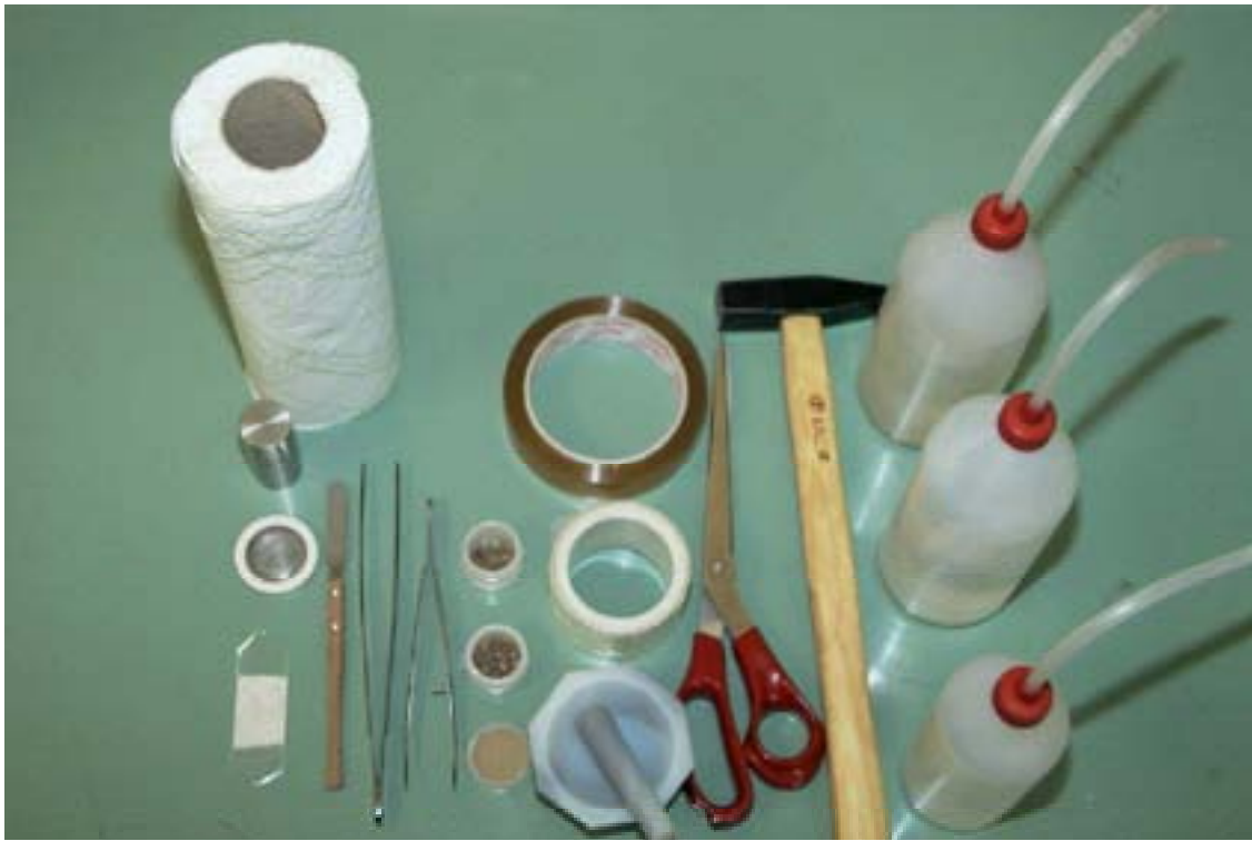
Fig. 9. Kit for sampling solid soil or geological samples.
