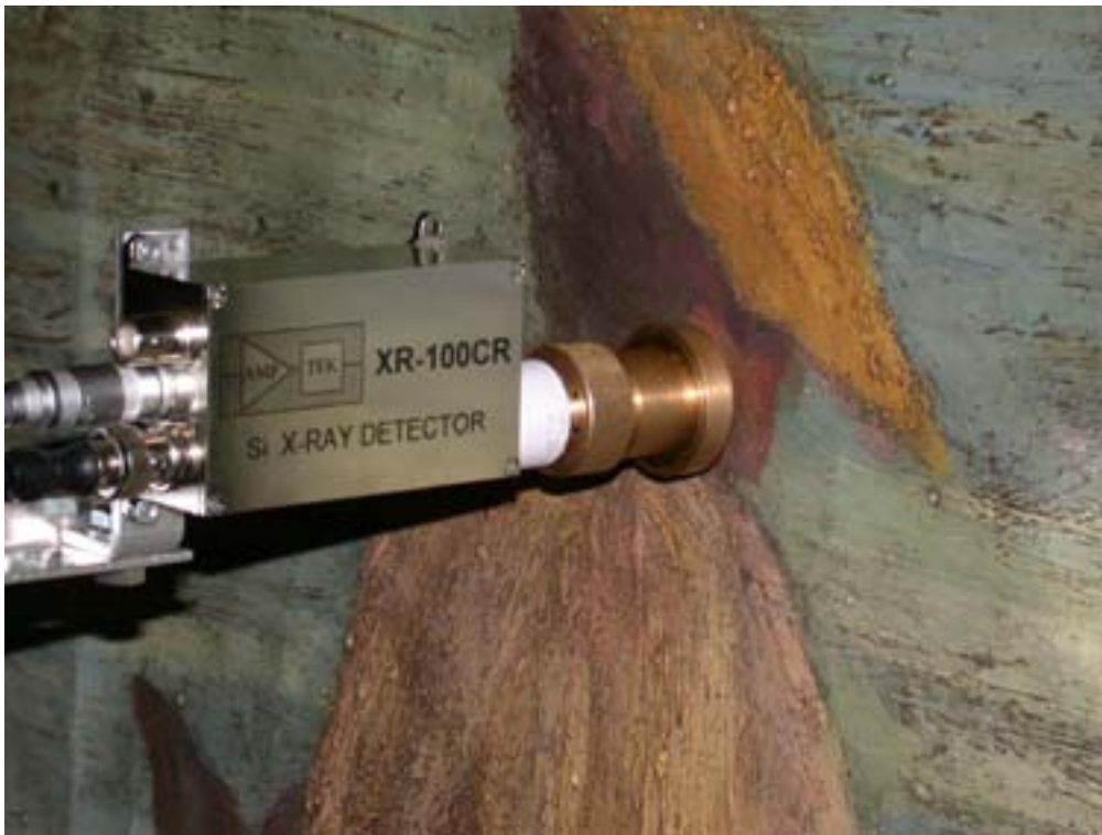
Fig. 4. The AMPTEK XR-100CR detector equipped with the ^{55}\text{Fe} excitation head.
