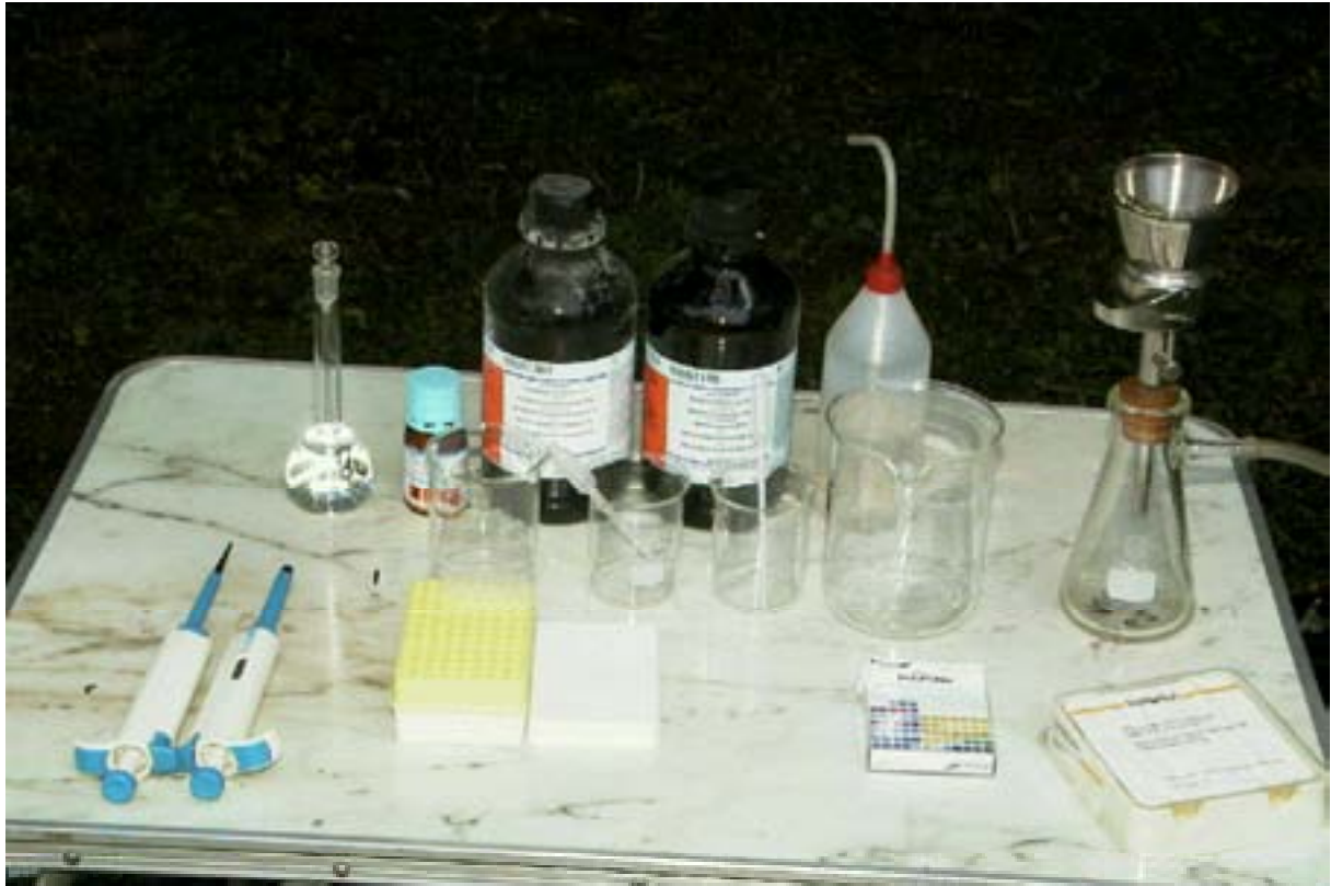
Fig. 12. Sample preparation kit for water sample precipitate.
