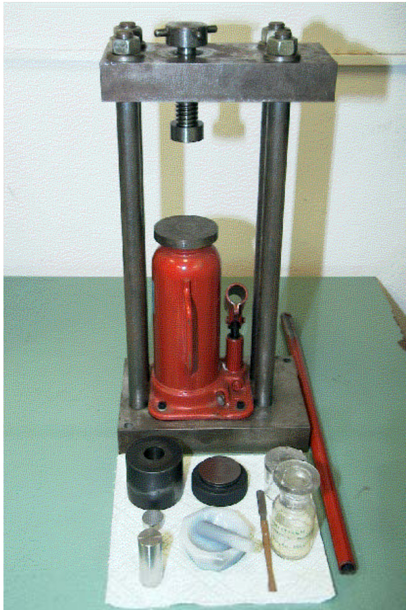
Fig. 10. Sampling kit for solid samples including pellet die and press.
