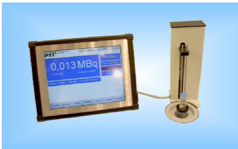
FIG. 20. Transport lift system for sample radioactivity measurement (Source: Wälischmiller GmbH, Germany).
