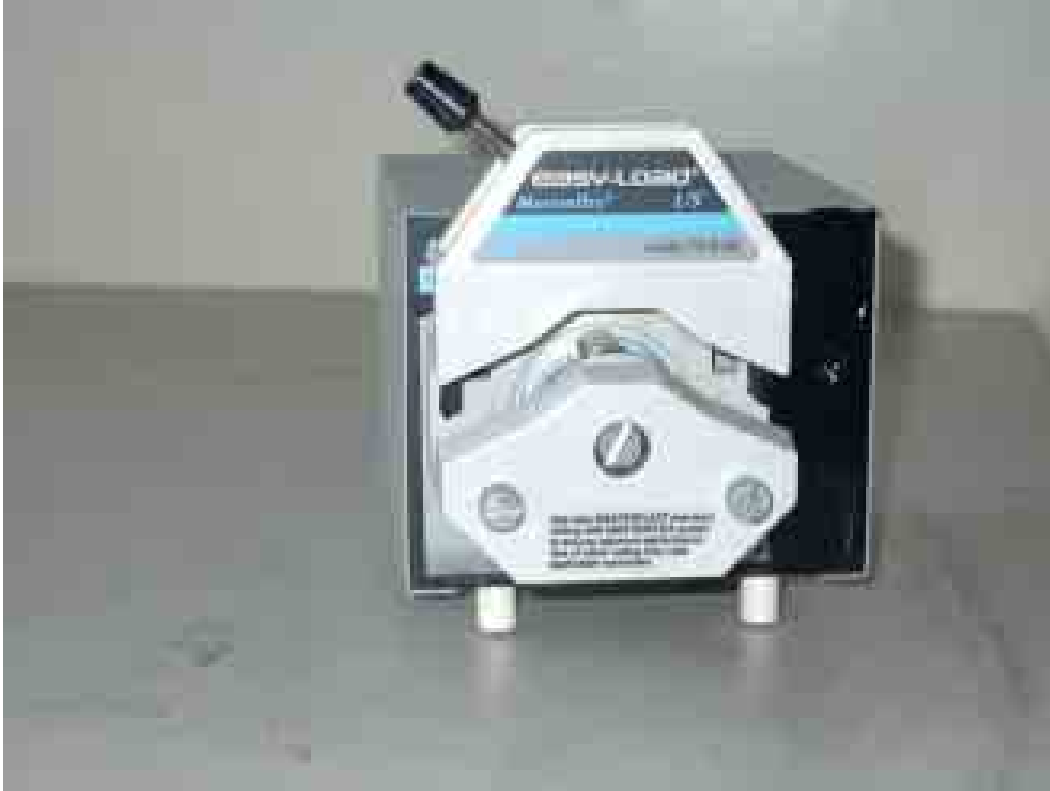
FIG. 19. Peristaltic pump operated with manipulator (Source: Commercially available).
