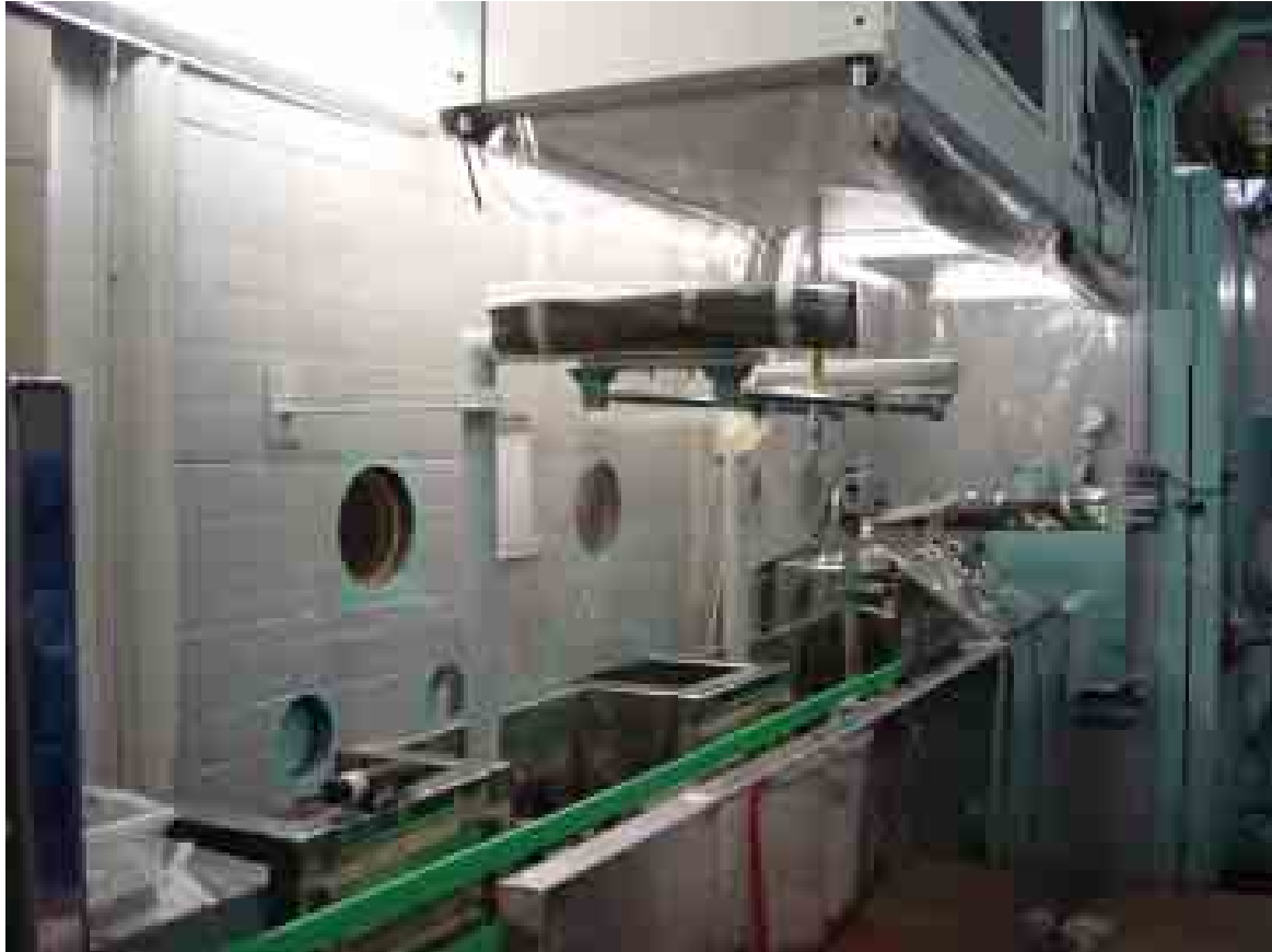
FIG. 29. ^{99}\text{Mo} - ^{99\text{m}}\text{Tc} generator production line (Source: IPEN, Brazil).
