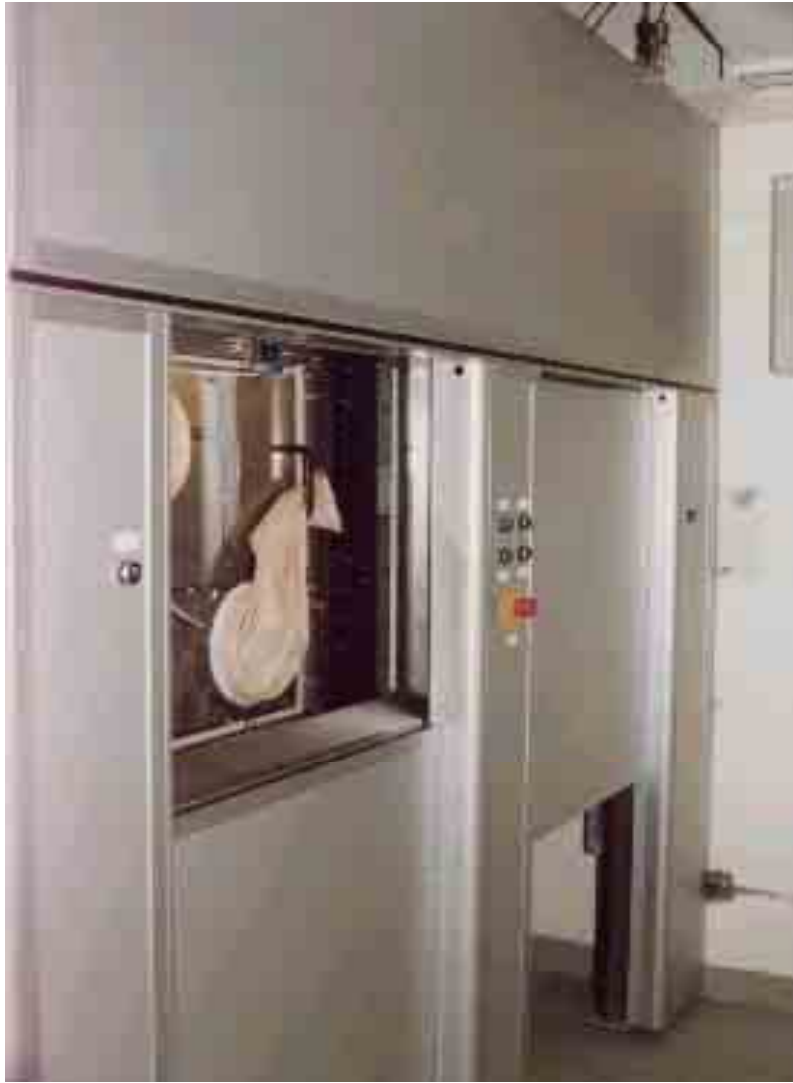
FIG. 8. Hot cell with openable rear wall (Source: Wälischmiller GmbH, Germany).
