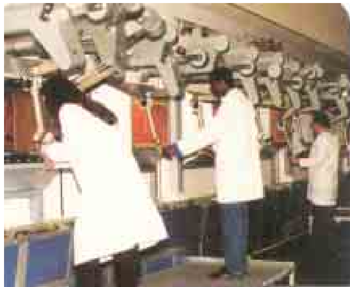
FIG. 7. Highly shielded hot cells with master slave manipulators (Source: NECSA, South Africa).
