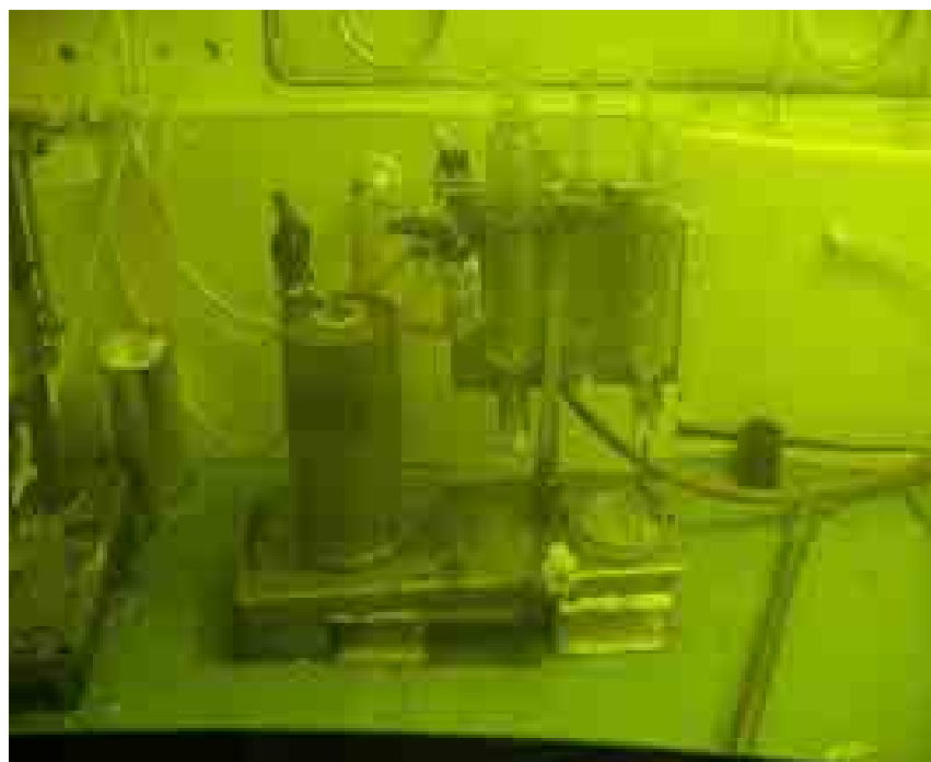
FIG. 21. Dry distillation equipment for ^{125}\text{I} production (Source: IZOTOP, Hungary).
