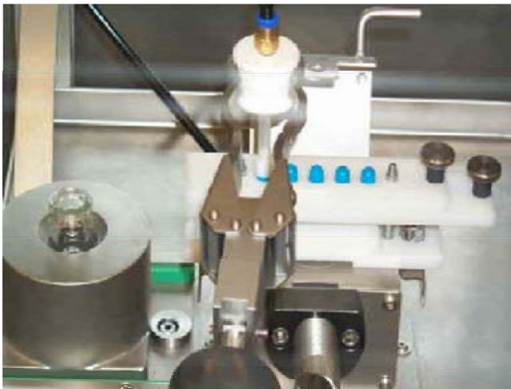
FIG. 3. In-cell equipment for Na 131 I capsule production (Capsules for diagnostic and therapeutic applications).
