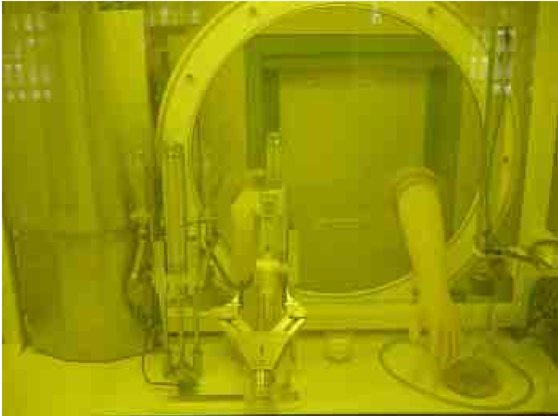
FIG. 32. FDG dispenser for use in isolator (Source: IPEN, Brazil).
