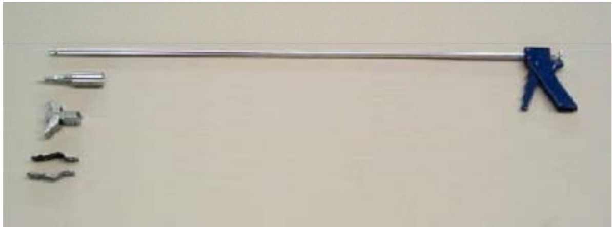
FIG. 12. Tong manipulator with accessories (Source: Wälischmiller GmbH, Germany).
