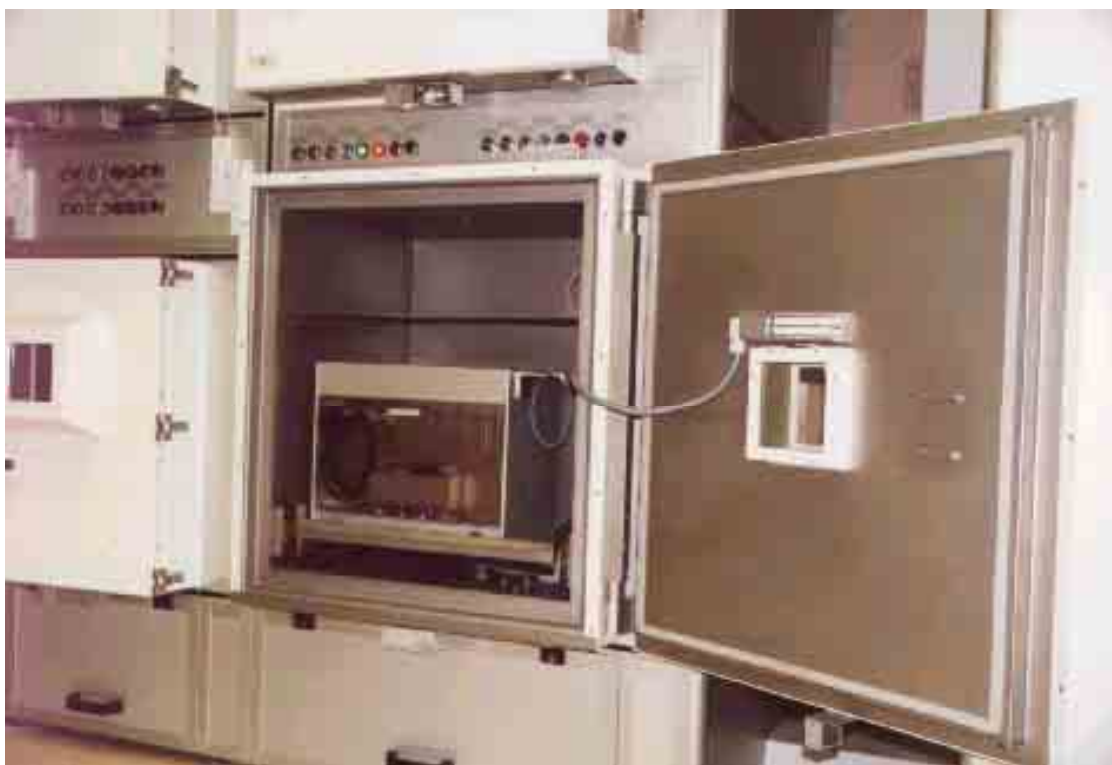
FIG. 33. Clean mini cell designed as isolator for PET-module operation (Source: Wälischmiller GmbH, Germany).
