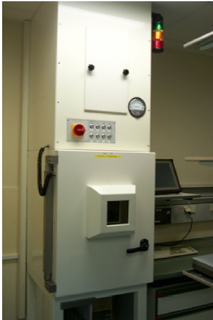
FIG. 9. Mini cell for dispensing with controlled air flow (Source: Wälischmiller GmbH, Germany).
