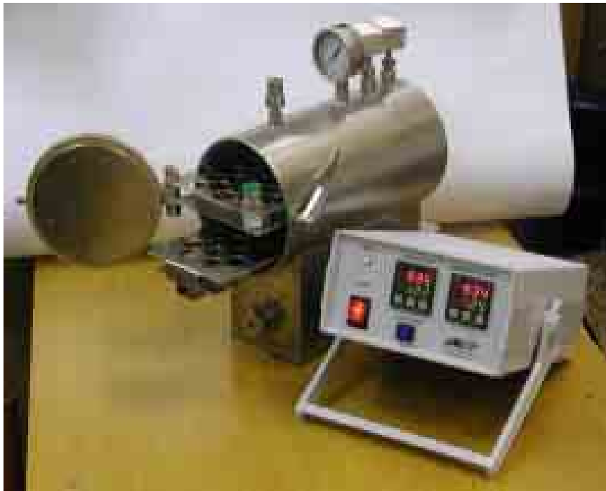
FIG. 17. Compact sized autoclave for ampoules (Source: IZOTOP, Hungary).
