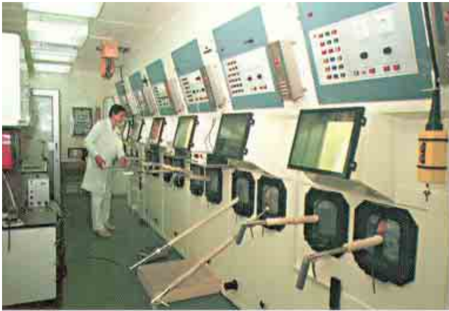
FIG. 3. Hot cell series with remote handling tongs (Source: IZOTOP, Hungary).
