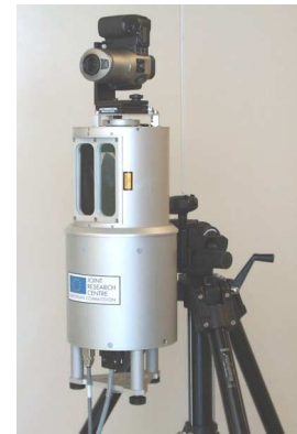
Figure 3: 3D Laser Range Scanner
