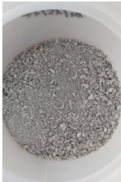
FIG. 24. Simulated incinerator ashes typical of combustible wastes (image courtesy of the University of Sheffield and the EU PREDIS Project).
