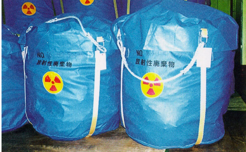
FIG. 29. Very low level waste placed in soft sided bags (image courtesy of the Japan Atomic Energy Agency (JAEA)).
