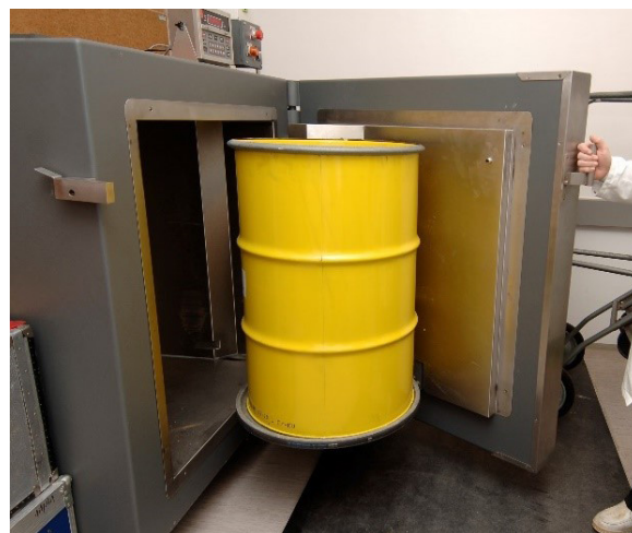
FIG. 31. A 200-L drum being placed inside a drum counter.
