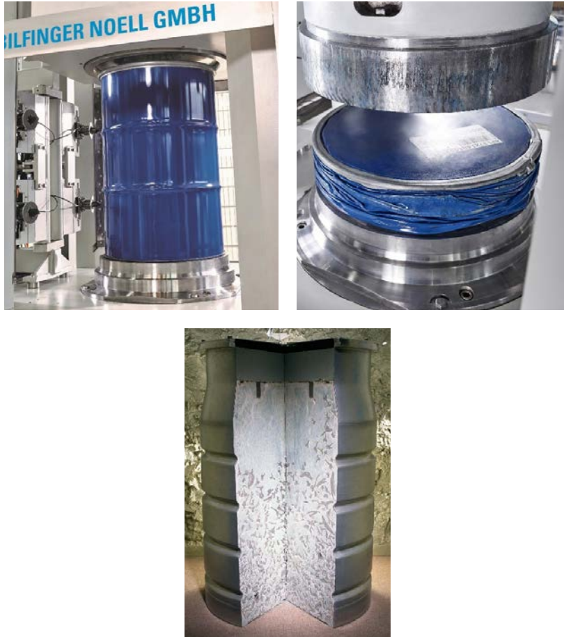
FIG. 16. Macroencapsulated waste examples. Top row: 200-L drum prior to (left) and after (right) supercompaction (image courtesy of Bilfinger Noell); bottom: Lillyhall 500-L ILW waste drum with cutaway (image courtesy of the Nuclear Decommissioning Authority, United Kingdom).
