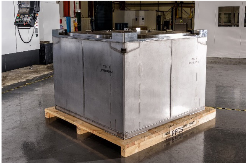
FIG. 33. Stainless steel box of 3 m 3 in size (image courtesy of Sellafield Ltd).
