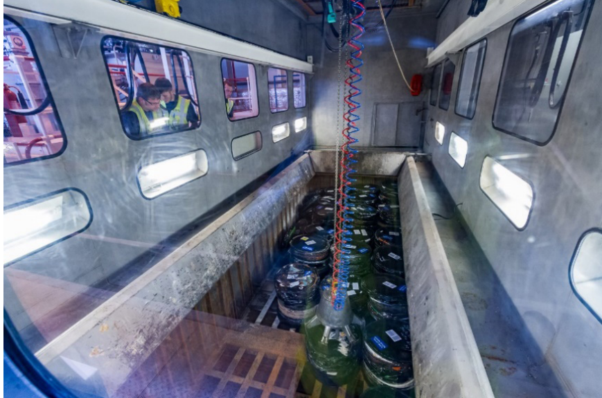
FIG. 27. LLW pucks loaded into a half-height ISO container overpack (image courtesy of Dounreay Site Restoration, Nuclear Decommissioning Authority, United Kingdom).
