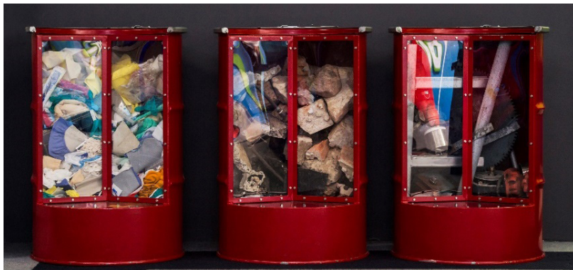
FIG. 14. A set of cutaway drums showing various types of solid LLW (image courtesy of the Australian Nuclear Science and Technology Organisation).
