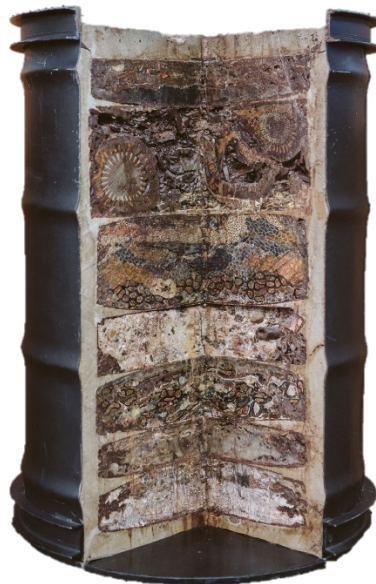
FIG. 28. Supercompacted primary drums overpacked in a secondary drum and immobilized with grout (image courtesy of ONDRAF/NIRAS).
