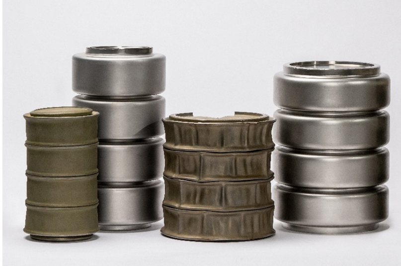
FIG. 20. ANSTO Synroc canisters, pre and post the hot isostatic pressing process (image courtesy of ANSTO).
