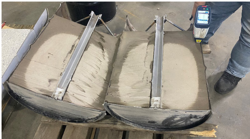
FIG. 17. Photo of a cementitious waste form (containing simulated waste) with a “lost paddle” design which has been cut in half to determine the homogeneity of the dispersed simulant material (tungsten); (image courtesy of United States Department of Energy/Idaho National Laboratory).
