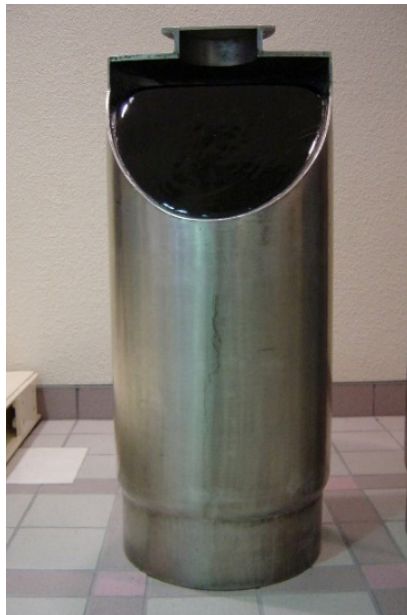
FIG. 19. Vitrified glass waste form in steel canister with cutaway to show interior glass (image courtesy of the Japan Atomic Energy Agency (JAEA)).
