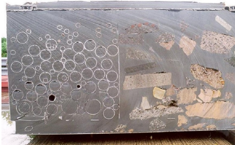
FIG. 15. Large format metallic and construction materials embedded in grout (image courtesy of Nuclear Decommissioning Authority, United Kingdom).
