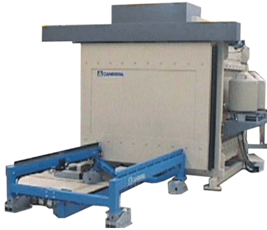
FIG. 12. A waste crate assay system for counting waste items and estimating nuclear material content (image courtesy of Mirion Technologies).
