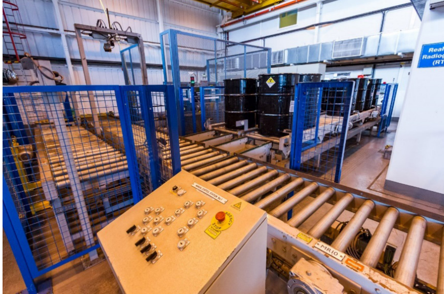
FIG. 25. LLW Drums entering the Dounreay Waste Receipt, Assay, Characterisation and Supercompaction (WRACS) facility (image courtesy of Dounreay Site Restoration, Nuclear Decommissioning Authority, United Kingdom).
