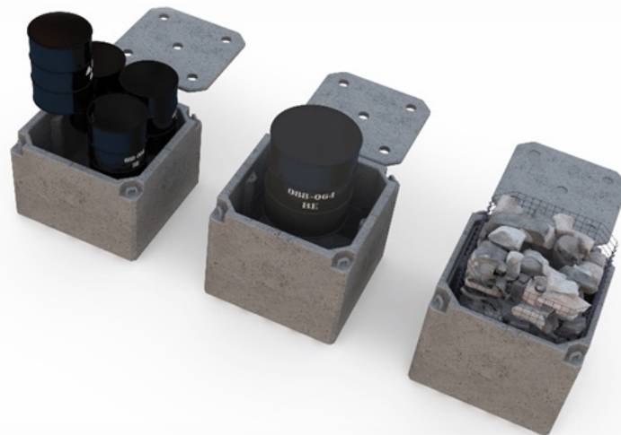
FIG. 32. Rendering of concrete boxes (caissons) showing various filling modes prior to final grouting. Examples include: multiple medium drums (left); one larger drum (centre); and large, loose components contained in an inset basket (image courtesy of ONDRAF/NIRAS).
