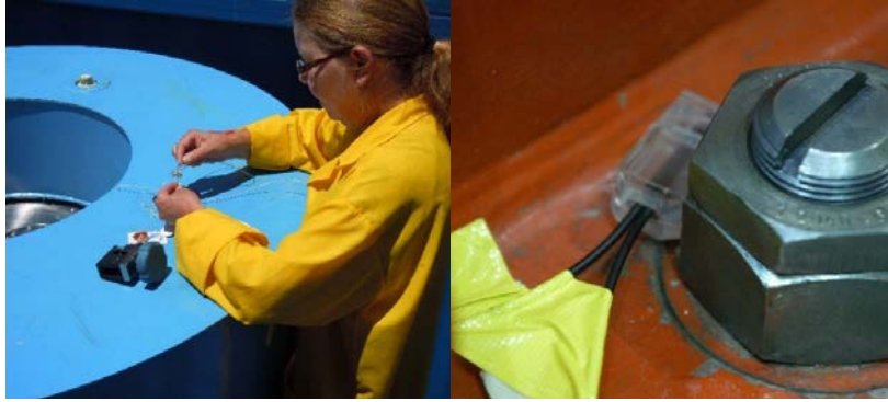
FIG. 9. Examples of seals that are used by the IAEA to maintain continuity of knowledge.
