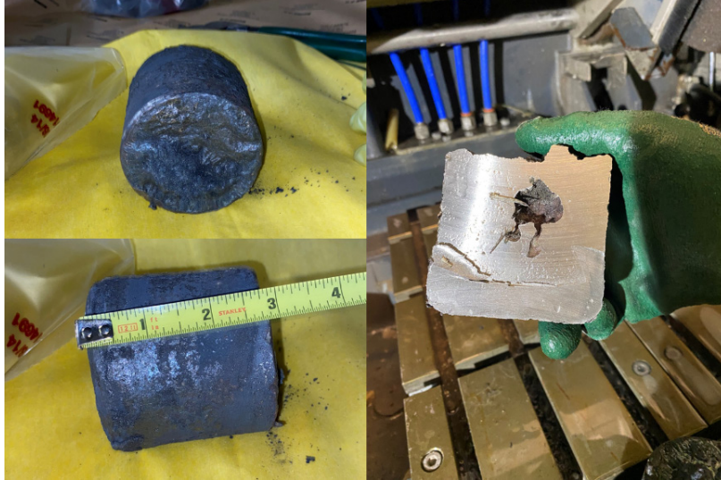
FIG. 18. Stainless steel–Yttrium–Uranium–Thorium metallic waste form, sectioned for characterization (image courtesy of United States Department of Energy/Savannah River National Laboratory).
