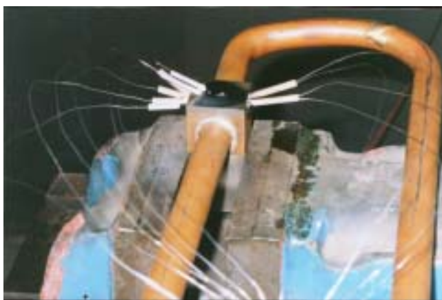
FIG. 4. Thermal load test at 10 \text{ MW m}^{-2} electron beam irradiation under 1000 cycles of 20 s duration and 20 s intervals for a W/CuCrZr weld by hot isostatic pressing.
