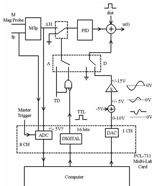
FIG. 1. Block diagram of the hybrid digital/analog feedback control circuit.
