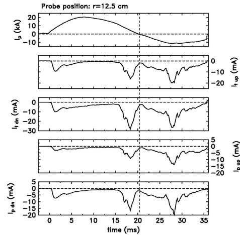
FIG. 4. Ion saturation currents on Mach probes at  $r=12.5$  cm (shot 135545).
