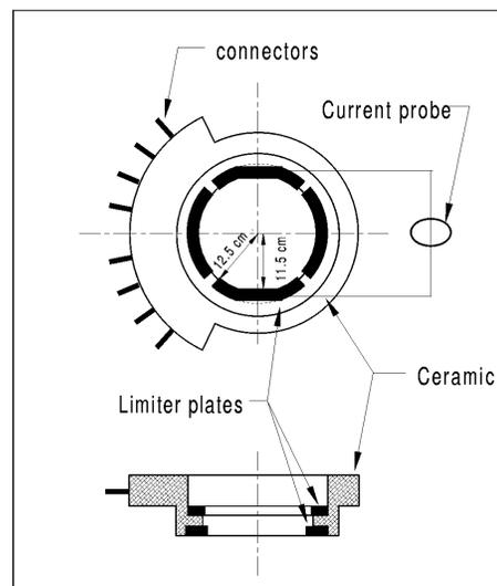
FIG. 2. Schematic diagram of the segmented limiter.
