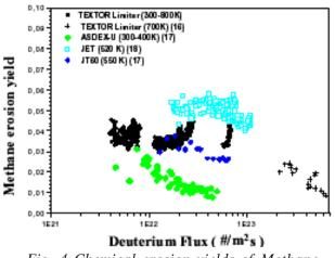
Fig. 4 Chemical erosion yields of Methane as a function of ion flux density.
