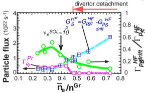
Fig.2 Particle fluxes towards HFS divertor,  $\Gamma_p^{HFS}$  and  $\Gamma_p^{Prv}$ , and ratio of drift flux,  $\Gamma_{p,drift}^{HFS}/\Gamma_{p,\ell''}^{HFS'}$  as a function of  $n_e$ . where the ion grad-B drift direction is towards divertor.
