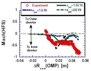
Fig. 3 Profiles of Mach numbers at HFS SOL (above HFS baffle): measurement (circles,  $n_e = 1.5 \times 10^{19} m^{-3}$ ) and simulations for three  $n_e$  scan.
