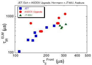
Fig.1 Energy deposition time from IRTV and characteristic time for ion flux to divertor form database (JET, ASDEX-U, JT-60U)
